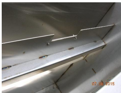
Figure 3-1b: Detail of adjustable overflow weir plate
