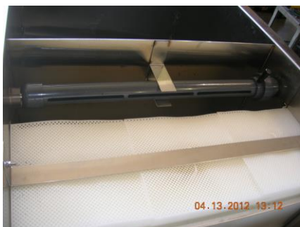
Figure 3-1a: Detail of PVC Pipe Skimmer
