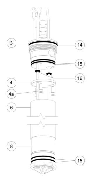
Figure 7-2: SS Geosub Pump, O-Ring Diagram
