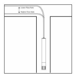
Figure 1-2: Minor Adjustments to Flow Rate
