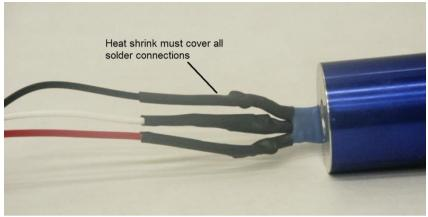
Figure 4-9: Heat Shrink Each Connection
