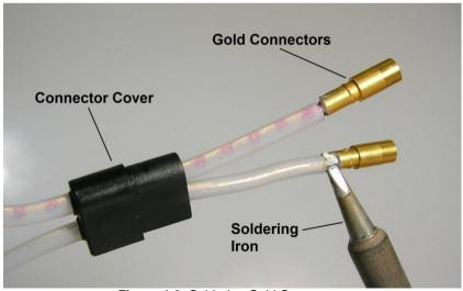
Figure 4-2: Soldering Gold Connectors
