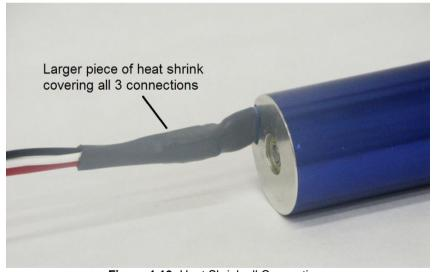
Figure 4-10: Heat Shrink all Connections
