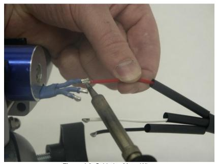
Figure 4-8: Soldering Motor Wires
