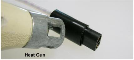
Figure 4-5: Heating the Heat Shrink
