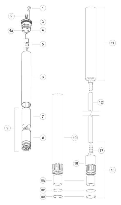
Figure 7-1: SS Geosub Pump and Drop Tube Assembly
