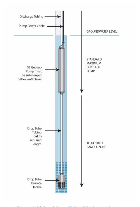
Figure 2-1: SS Geosub Pump with Drop Tube Assembly in well
