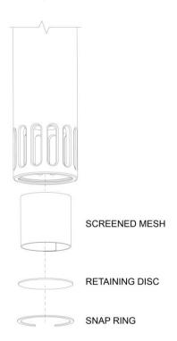
Figure 4-1: Screened Intake Components
