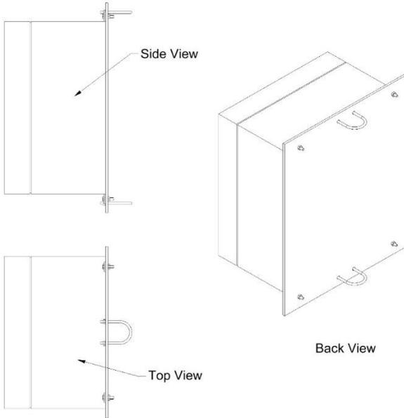
**Figure 2-4:** Example of pole mounting enclosure
