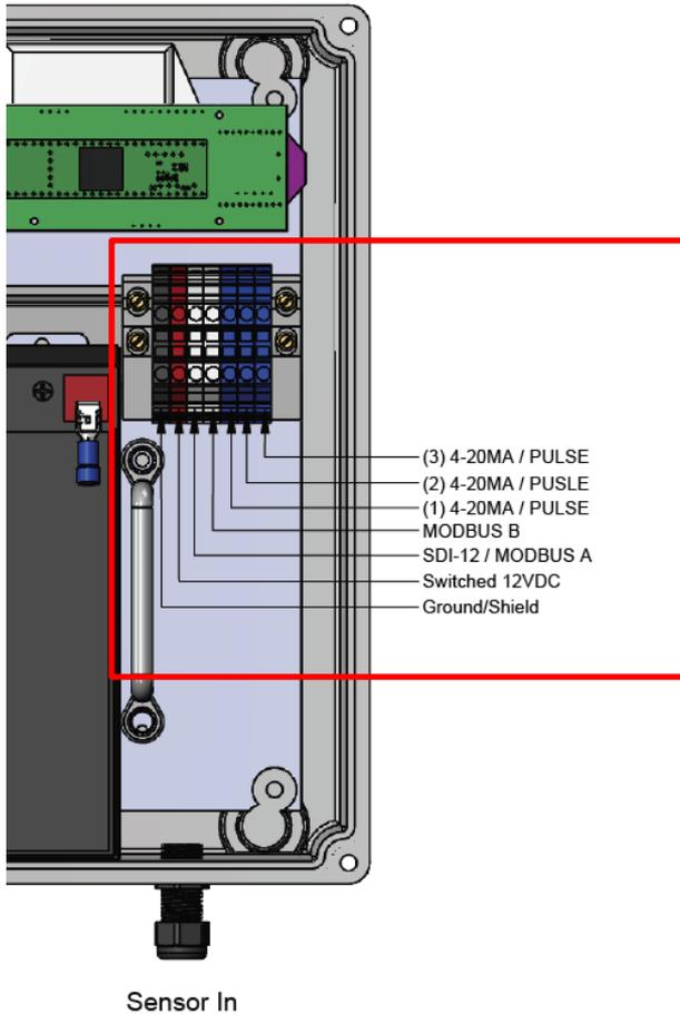
**Figure 2-7:** Sensor connections to terminal strip
