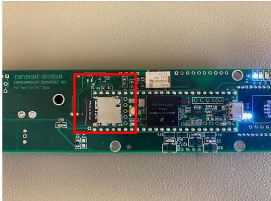
**Figure 4-1:** SD Card on PCB
