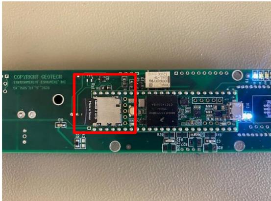
**Figure 4-1:** SD Card on PCB
