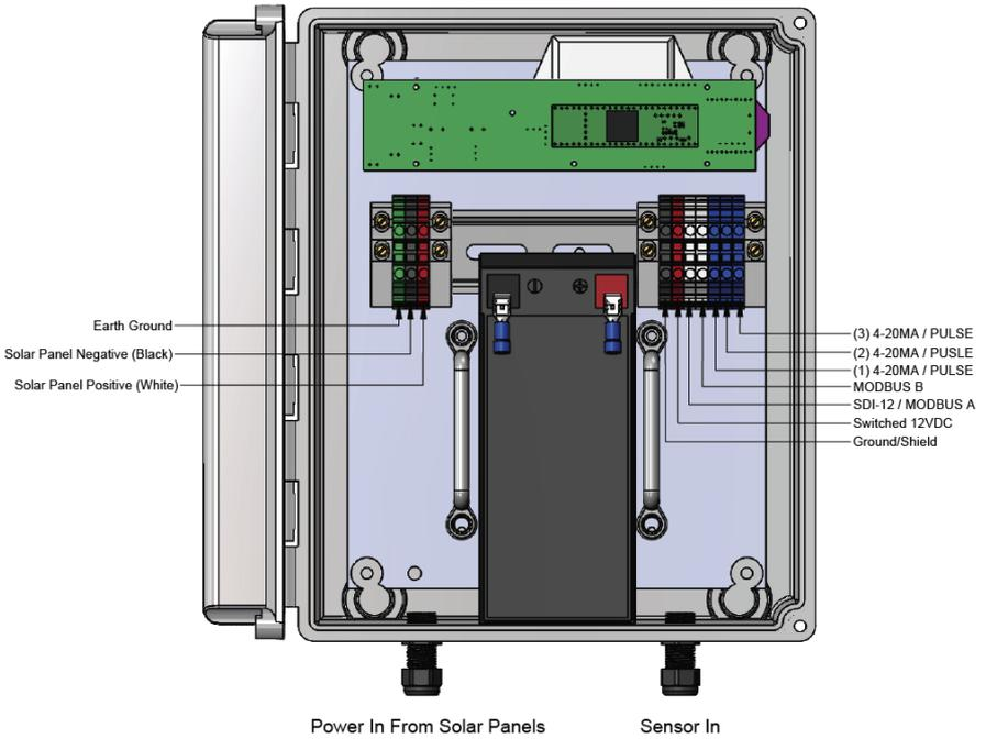
**Figure 7-1: Solar Panel and Sensor Input Wiring**
