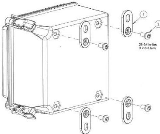
**Figure 2-5:** Example of panel mounting enclosure
