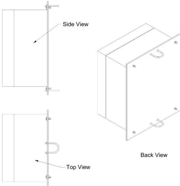
**Figure 2-4:** Example of pole mounting enclosure
