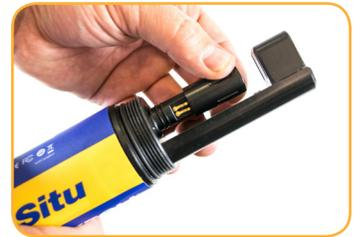
Align the slotted edge of the RDO cap with the flat edge of the RDO sensor. Press the cap firmly into position.
