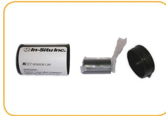
Locate the RDO sensor cap container and remove the cap.
