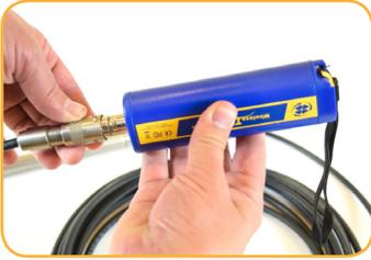
Connect Rugged Cable to the Wireless TROLL Com and instrument.
