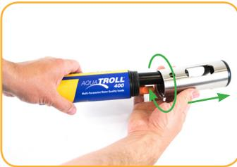
Twist the restrictor off the probe.
