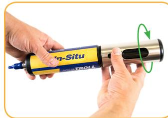
Twist the restrictor back onto the probe.
