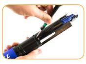
Lever the Allen wrench towards the top of the sonde to slide the sensor out.
