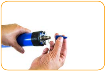
Remove protective caps from instrument and cable.
