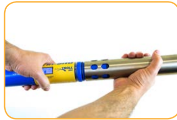
Replace restrictor with vent holes at base of instrument.
