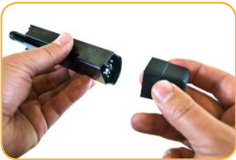
Remove dust cap from pH/ORP sensor.
