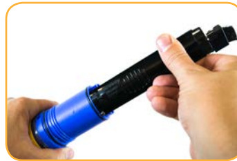
Install sensor in port 1. Sensor tongue must slide into blue interlock groove.
