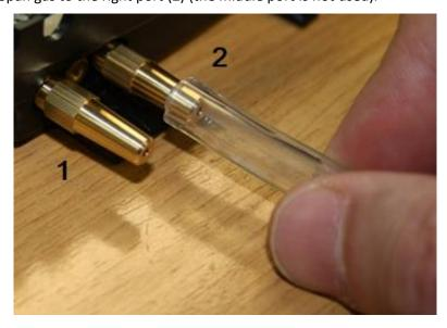
• The Zero and Span times are affected by the length of pipe between the gas source and the Calibration Dock. For best results, ION Science recommends that pipe lengths should be kept to a minimum; the shorter the length, the less gas is needed.
