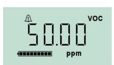
If the detected gas level triggers a low-level alarm, the display screen will flash orange, and the lights on the top of the unit will flash red.
