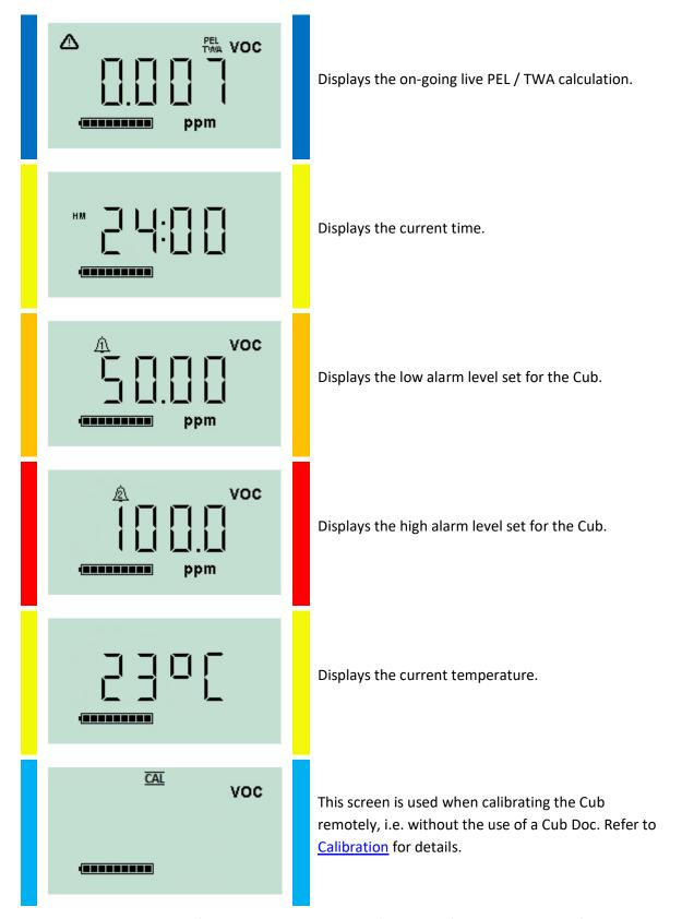
Note that a Cub can be configured to only display specific screens (see the <u>Device Configuration</u> section for details.
