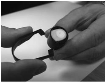
Using the Mini PID Electrode Stack Removal Tool provided, locate its 'prongs' in the slots in the side of the Mini PID 2 Sensor Body.
