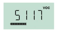
The screen will change and display a live reading from the sensor. *This number does not relate to gas concentration*, it simply indicates if the sensor output is changing.
