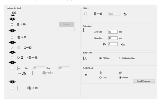
This page is used to set preferences for the CubPC software, such as actions taken when Cubs are docked.
