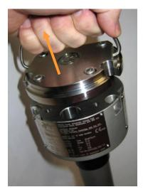
If this procedure is not followed carefully, damage to the O-ring may be caused compromising the intrinsic safety of the Unit.
