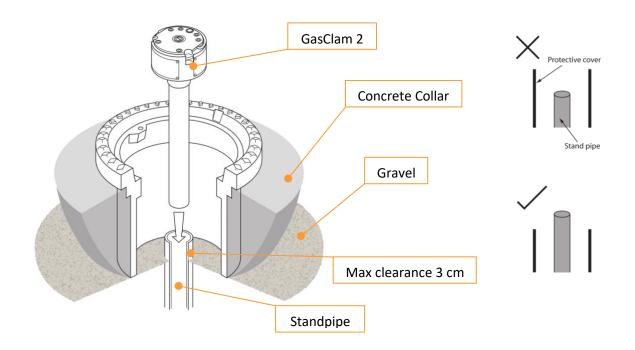
It is important to have the standpipe a maximum of 3 cm above the base of the Headworks, this will ensure the GasClam 2 will fit under the lid of the cover. The Headworks must be concentric to the standpipe for the GasClam 2 to be housed correctly. The standpipe must also be cut square to allow a good seal.
