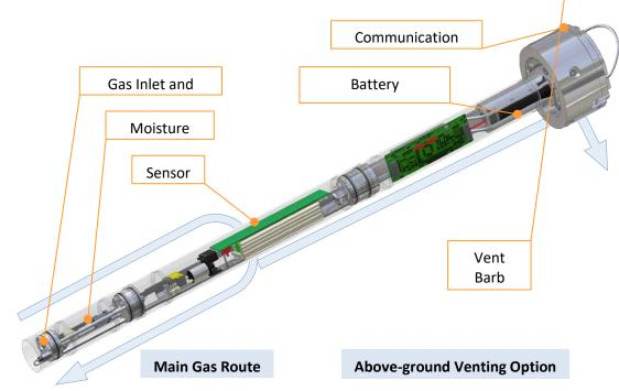
When logging is started the GasClam 2 instantly takes its first sample. A click is heard and then the pump starts which takes a sample of air from the borehole. First the pressure and temperature readings are taken. While the pump is on readings from gas flow sensors are taken. The pump then switches off and after a short pause readings from static gas sensors are taken. The whole process takes approximately 2 ½ minutes depending on sensor configuration.
