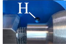
(Flame Arrestor Cap assembly is located on the side of the enclosure)
