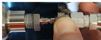
5. Turn the red handle 180° to open valve. The arrow should point toward the fill hose.
