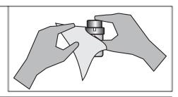
Open the meter lid. Insert the tube into the chamber. Align the index notch on the positioning ring with the index arrow on the meter. Close the lid.
