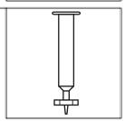
Remove the filter from the syringe. Remove the plunger from the barrel. Replace the filter and fill the syringe with approxiamtely 50 mL of deionized water. Filter the water into the storage conatiner and save this turbidity-free water.
