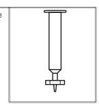
2. Pour approximately 50 mL of deionized water into the barrel of the syringe. Insert the plunger. Exert pressure on the plunger to slowly force the water through the filter. Collect water in the clean storage container. Rinse walls of the container then discard this rinse water.
