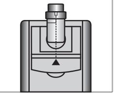
7. Press \*IOK to select Scan Blank. Remove the tube.
