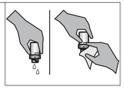
Fill the tube to the fill line with the standard. Pour the standard down the inside of the tube to avoid creating bubbles. Cap the tube.
