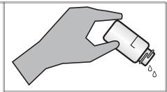
4. Fill the tube to the fill line with the blank. Pour the blank down the inside of the tube to avoid creating bubbles.
