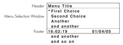
An asterisk, \*, will start in the far left position of the top line in the menu choice window. To move the \* press the up or down arrow buttons (▲ or ▼) to scroll through the menu selections. The \* in the display corresponds with the \*IOK button. Pushing the \*IOK button selects the menu choice which is adjacent to the \* in the menu selection window.
