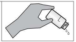
4. Fill the tube to the fill line with the blank. Pour the blank down the inside of the tube to avoid creating bubbles. Cap the tube.
