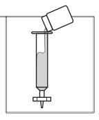
3. Remove the filter from the syringe. Remove the plunger from the barrel. (This step is required to prevent rupturing the filter by the vacuum that would be created when the plunger is removed.)
