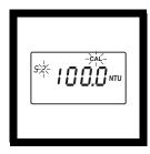
10. The display will show the S2 icon (with the 2 flashing) and 100 NTU or the value of the S2 standard for the previous calibration.
