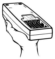
**2.** Remove the lamp assembly by grasping the tab on the left side of the assembly. Firmly, but gently, slide the assembly towards the rear of the instrument.
