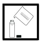
**1.** Fill a clean sample cell to the line (about 15 mL) with dilution water.
