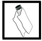
**2.** Wipe the cell with a soft, lint-free cloth to remove water spots and fingerprints.
