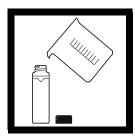
1. Fill a clean sample cell to the line with clear water, cap the cell and place it in the cell compartment. Press the READ key and wait until the reading is finished.
