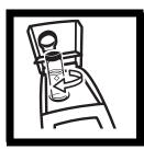
**5.** Remove the cell, rotate it slightly and reinsert it into the cell compartment. Close the cover, then press **READ**. Record the cell's position and the displayed reading.
