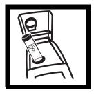
**4.** Place the 0-10 NTU Gelex standard in the cell compartment so the diamond on the vial aligns with the orientation mark on the instrument. Close the sample lid.
