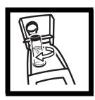
**8.** Remove the cell, rotate it slightly and reinsert into the cell compartment. Close the cover, then press **READ** again. Record the cell's position and the displayed reading.
