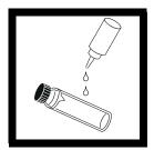
**3.** Apply a thin film of silicone oil. Wipe with a soft cloth to obtain an even film over the entire surface.
