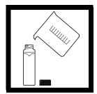
1. Rinse a clean sample cell with dilution water several times. Then fill the cell to the line (about 15 mL) with dilution water or use StablCal <0.1 NTU standard.
