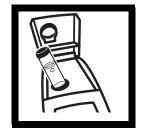
**6.** Repeat *step 3* through *step 5* for the other Gelex standards, being careful to orient the cells properly.
