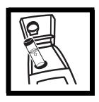
**6.** Insert the **second** sample cell into the cell compartment and close the cover.
