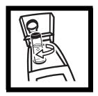
**9.** Repeat *step 8* until the value displayed for the second cell is within 0.01 NTU (or 1%) of the value obtained for the first cell. Place an orientation mark on the second cell's marking band so it is consistently inserted in this position.
