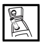
**4.** Insert the **first** sample cell into the sample compartment and close the cover.
