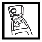
**6.** Repeat *step 5* until the lowest reading is displayed. Place an orientation mark on the cell's marking band near the top of the cell so the cell can be consistently inserted in the position that yields the lowest reading. When using the cell, always place it in the instrument so the orientation mark aligns with the raised mark on the instrument
