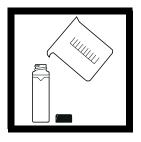
1. Fill the clean sample cell to the line with high quality water (< 0.5 NTU). Cap and wipe with lint-free cloth. Apply silicone oil. See Section 3.6.2.2 on page 40 for more information about high quality water.
