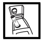
**3.** Insert the sample cell into the sample compartment. Close the cover.
