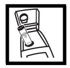
9. Thoroughly mix the 90 to 110 NTU standard, then fill a clean sample cell to the line with the standard. Insert the cell into the cell compartment.
