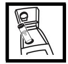
2. Insert the sample cell in the cell compartment by aligning the orientation mark on the cell with the mark on the front of the cell compartment. Close the lid Press I/O.
