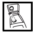
2. Insert the sample cell into the cell compartment and close the lid. Press I/O.
