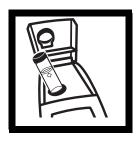
13. Thoroughly mix the 700 to 900 NTU standard, then fill a clean sample cell to the line with the standard. Insert the cell into the cell compartment.
