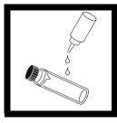
**2.** Apply a small bead of silicone oil from the top to the bottom of the cell-- just enough to coat the cell with a thin layer of oil
