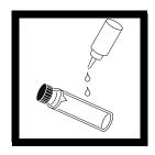
**3.** Thoroughly clean the outside of the Gelex vials and apply a thin coating of silicone oil.
