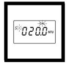
**6.** The display will show the **S1** icon (with the **1** flashing) and **20** NTU or the value of the S1 standard for the previous calibration.
