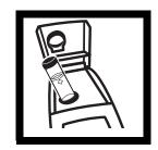
5. Thoroughly mix the 10 to 30 NTU range standard, then fill a clean sample cell to the line with the standard. Insert the sample cell into the cell compartment
