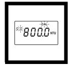
14. The display will show the S3 icon (with the 3 flashing) and 800 NTU or the value of the S3 standard for the previous
