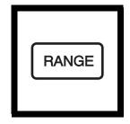
**6.** Select manual or automatic range selection by pressing the **RANGE** key. The display will show **AUTO RNG** when the instrument is in automatic range selection.
