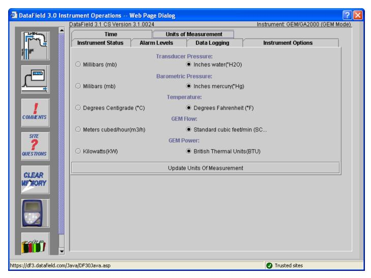
**Note:** EXTREME CAUTION should be taken if changing the Units of Measurement. All data from the instrument should be downloaded and stored in both, the GEM and the GA modes before updating the Units of Measurement. Updating Units of Measurement will erase readings from the instrument. The instrument should be turned off and restarted once the units of measurement have been updated.
