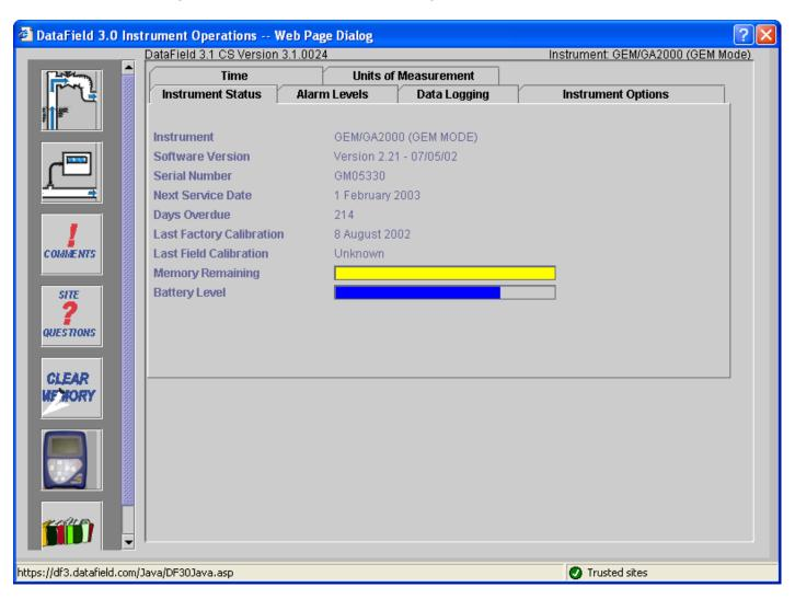
There are six different "Menu Cards" under instrument settings. Each card provides different information or instrument settings that may be changed to update the operation of the GEM™2000. The instrument status card will always be shown first, providing calibration and maintenance information in addition to instrument serial number and software version number.
