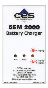
The battery charger indicates when the unit is charging, charged or if there is a fault. A full charge should take approximately 2 hours. Charge the batteries until the 'Charging Complete' indicator is flashing.
