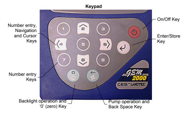
Whenever a key is pressed the unit will emit a short 'beep' as an acknowledgement. This function cannot be turned off.
