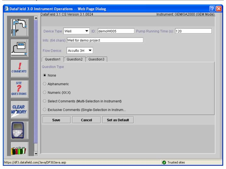
When editing is completed, click on **Save** to return to the previous screen. Click on **Save File** to save the edited data to disk or click on **Send to Instrument** to append the IDs to the IDs in the instrument.
