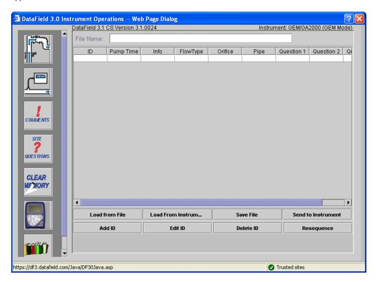
Seven main categories (buttons) are listed down the left side of the screen: ID Functions, Readings, Comments, Site Questions, Clear Memory, Instrument Settings and Resource Links. Clicking on any one of the buttons will take the user to that functionality of the application.
