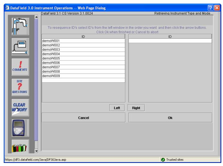
Select the ID from the left side window and click on the **Right** button to move ID to the right window to create the new sequence order. Repeat this process moving all IDs to the right side in the desired order.
