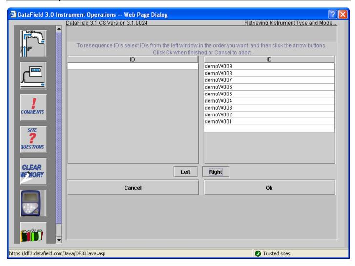
Click OK when the desired new sequence is obtained, this will return you to the well ID screen. Click on the **Save File** button to save the new data set to a file on disk or click on **Send to Instrument** to upload the new data to the instrument.
