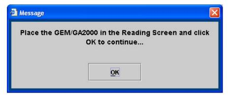
Click OK and DataField CS will automatically search for the instrument. This may take a few minutes. When the instrument is found and the communication is established, the software will display a box that indicates what type of instrument was found. If the software does not find the instrument, it will display a box that indicates that no instrument was found.
