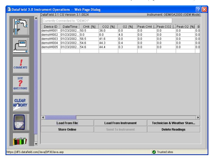
Once the file has been opened or data downloaded from the instrument, the readings can be either **stored online** (only with the online version) or **saved to a file** (only with the offline version). When the instrument is in the GA Mode the readings can also be **sent to the instrument**. **Send to Instrument** button will be disabled when the instrument is in the GEM Mode. The screenshot above shows the online version with the instrument in the GEM mode.
