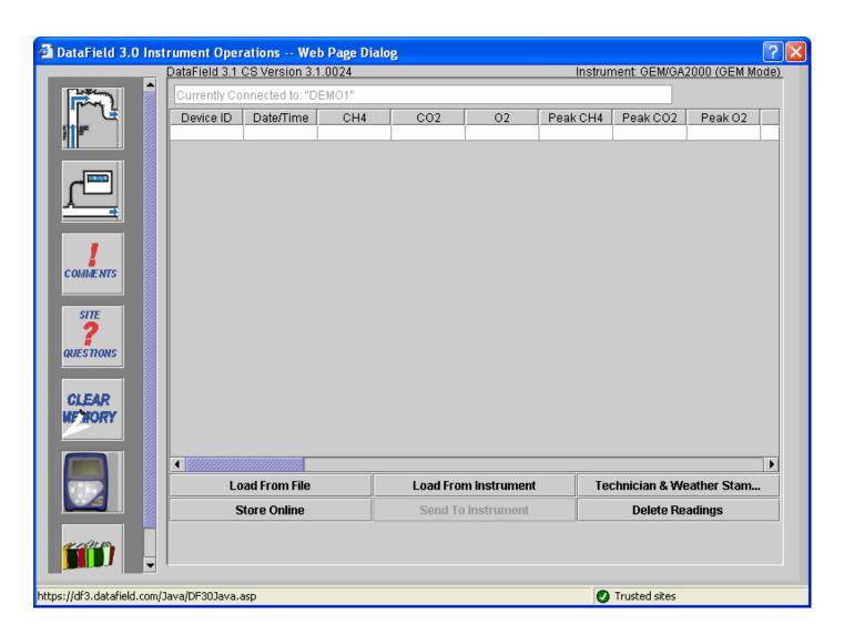
Click on **Load from File** to open a file folder of saved data on the disk drive or click on **Load from Instrument** to download data from the instrument. Either action will open the following screen. All readings should be downloaded on a daily basis. While the instrument can hold readings for an extended period of time, it is recommended to download them to a non-volatile memory device (e.g. hard drive, CD, etc.).
