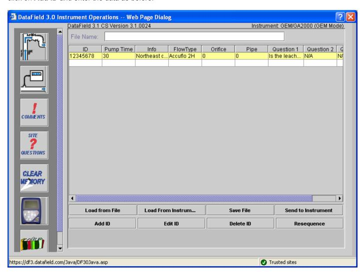
Once all the IDs have been entered, click **Save File** button to save the ID data to a file or **Send to Instrument** button if data is to be uploaded to an instrument for field sampling.
