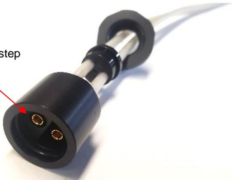
16. Push wire seal into housing cavity.
