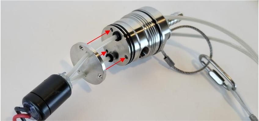
8. Secure bottom cap in place using the three (3) 6-32 x 3/8 screws.
