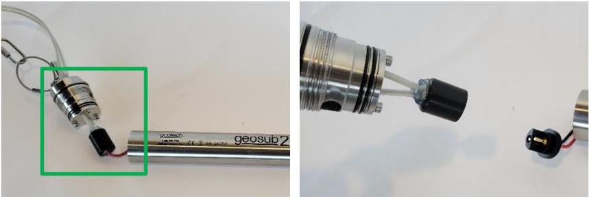
5. Use an appropriate tool to lightly twist and then pull the motor impeller, to remove it. The Geosub 2 assembly/disassembly tool is recommended to avoid damage to the impeller or internal wires.
