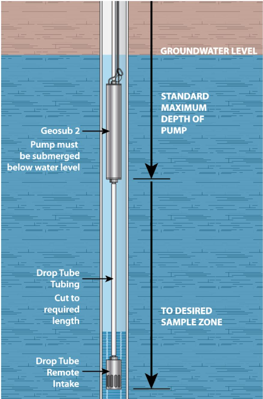
**Figure 2-1:** Geosub 2 Pump with Drop Tube Assembly in Well
