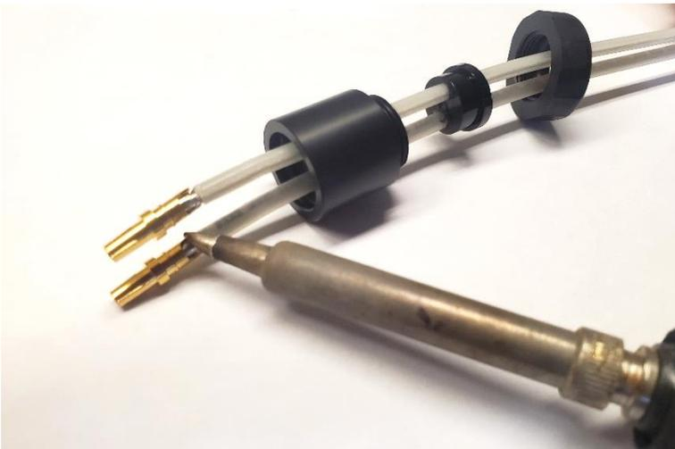
15. Pull wires back through housing so that the pins are slightly below the step.
