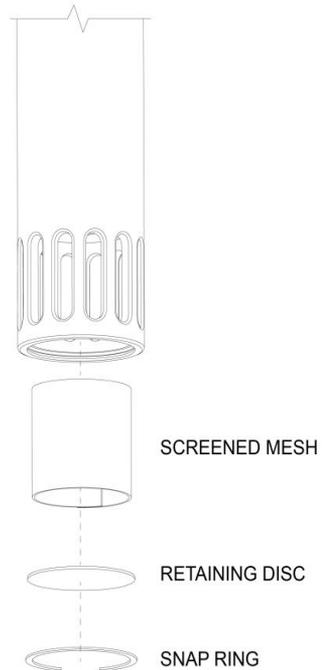
**Figure 4-1: Screened Intake**
