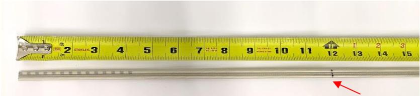
3. Using an X-acto blade (or similar blade), score the cable between safety cable and conductors, on each side of the safety cable.
