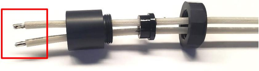
14. Solder wires to female pin to the stripped wires.
