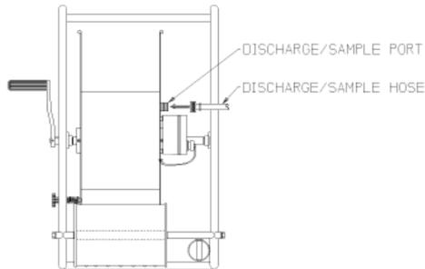
Figure 6: Discharge Ports
