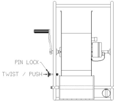
Figure 9: Pin-locking the Reel
