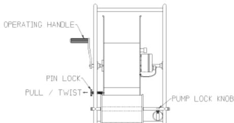
Figure 3: Unlocking Pump Holster Pin
