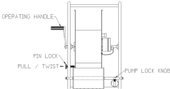
Figure 8: Unlocking the Pin Lock
