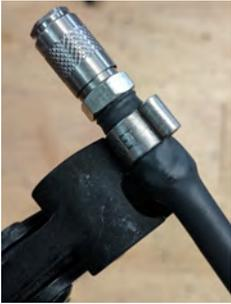
2. *Grasp* the other “ear” of the **Pinch clamp** with the **Angled High Leverage Cutters (LDAR#4234)**.
