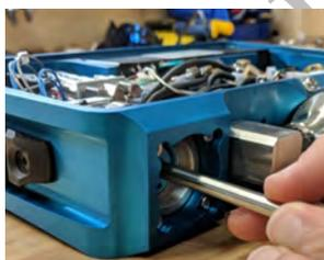
9. If necessary, slightly *rotate* the tool until the pins line up. Once they do, lightly *push* the **glow disk** into position.
