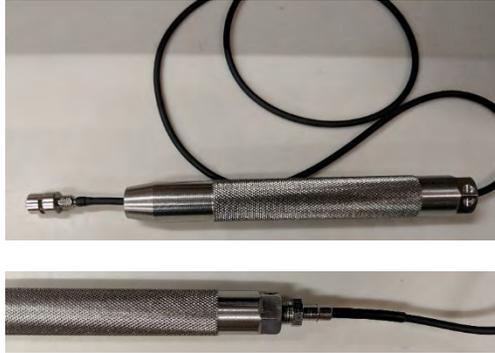
5. Slide 2 inches of the **Small Heat Shrink (LDAR #42087)** over the **Tubing** until about 1 inch is inside of the **Handle** and about 1 inch is still visible.
