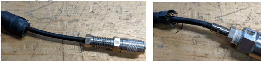
8. *Pull* the **Tubing (LDAR#42083)** off of the barb on the Quick Disconnect end.
