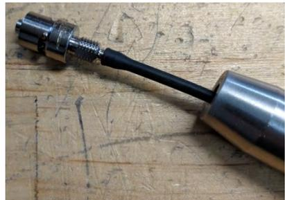
11. *Pull* the Tubing off of the barb of the fitting.
