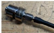
3. *Feed the other end of the tubing all the way through the center of the Handle (LDAR #42081) until you can thread the Male Luer bulkhead into the Handle.*
