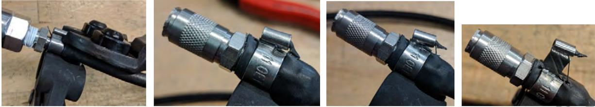
5. Pull the cut clamp off with the **Pinch Clamp Plier** by pulling on the remaining “ear” of the clamp that you were already gripping.
