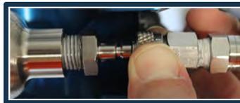
5. Confirm that the **H<sub>2</sub> fill adapter** is firmly seated on the **H<sub>2</sub> fill port**.
