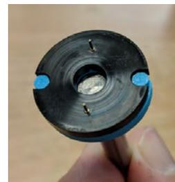
7. *Look* inside the **FID housing** to check the orientation of the sockets that the **glow disk** will plug into.
