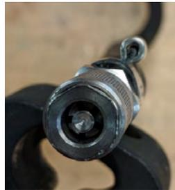
Before squeezing with **Angled High Leverage Cutters**      After squeezing with **Angled High Leverage Cutters**
