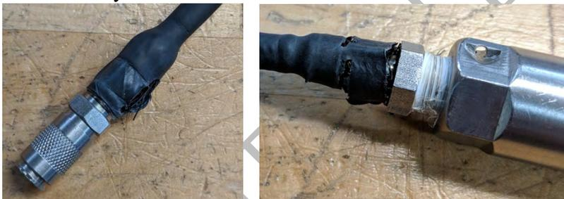
7. Once both Pinch Clamps are removed, pull off the outer **Large heat shrink (LDAR#42094)** and **Sheath (LDAR#42082)** using the **Angled Wire Cutters (LDAR#1741)** if necessary.
