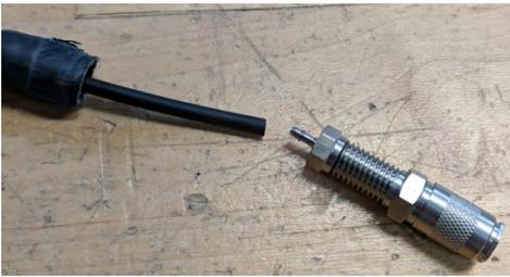
9. On the base of the probe, *pull* the **Tubing (LDAR#42083)** out and *cut* it off above the **Heat Shrink**.
