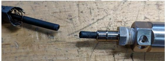
10. *Unthread* the **Luer lock** fitting at the tip of the **probe**. Try first with fingers alone. If this does not work, gently grip the fitting in the notch with the crimping pliers and loosen. Be careful to avoid the central stem of the fitting since this is the sealing surface.
