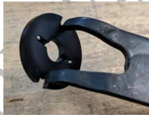
5. Pull the **glow disk** straight out to remove it from the **flame arrestor housing**.
