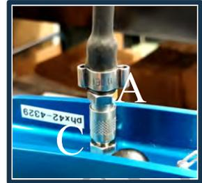
**REMINDER:** The **probe** and a **probe tip filter** should be connected to the **phx42** before igniting the device (unless performing filter detection calibration).
