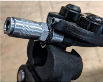
3. *Squeeze* the **Angled High Leverage Cutters** on the “ear” to get it ready for cutting.
