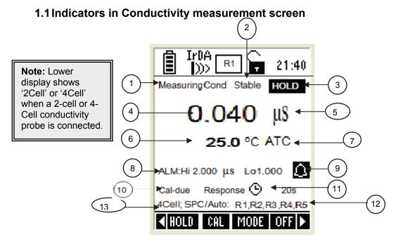
Figure 28 : Conductivity measurement screen
