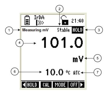
Figure 16: mV measurement screen
