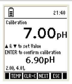
1. Rinse the electrode in clean water and prepare electrode for calibration.
