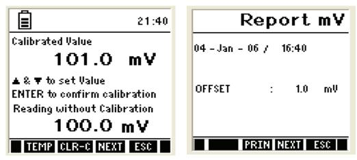
Figure 15: mV calibration screen & calibration report
