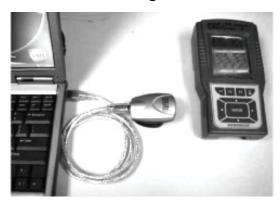
You can purchase an USB/ irDA dongle 01X447601 (see accessories page at the back of this manual) and transfer data from your meter using the USB port.
