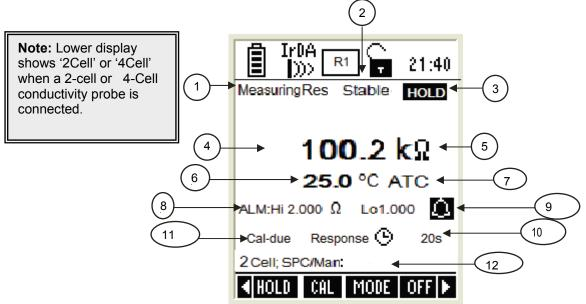
Figure 42: Resistivity measurement screen
