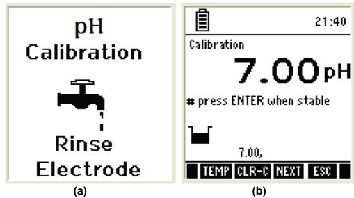
Figure 13: pH Calibration Screens
