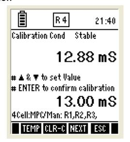
Figure 25: Conductivity calibration Screen
