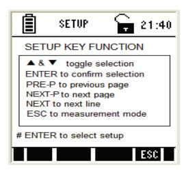
**Note:** If the meter is password protected, you will be prompted to enter a password before accessing Setup Key Function screen.
