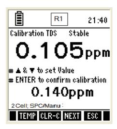
Figure 31: TDS Cell constant adjustment & TDS calibration screen
