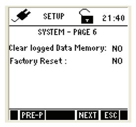
This allows you to clear the memory and reset the meter to factory defaults.
