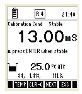
Figure 26: Conductivity calibration Screen-Auto
