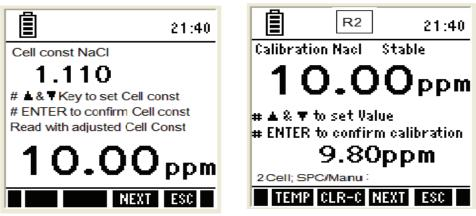
Figure 35 : Salinity Cell constant & salinity calibration
