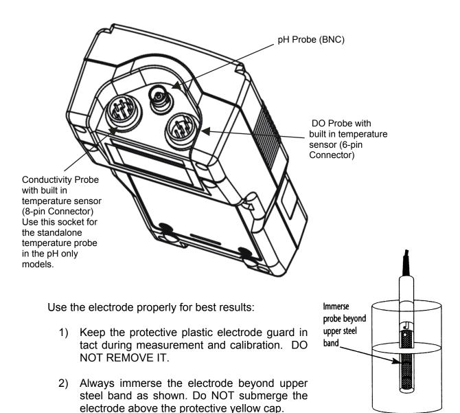
3) Be sure to remove the protective electrode storage bottle or rubber cap of the pH electrode before calibration or measurement.
