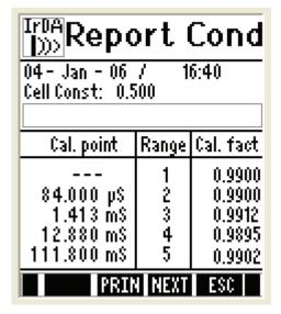
Figure 27: Conductivity Calibration Report
