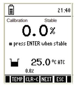
Figure 47:0% saturation calibration Screen
