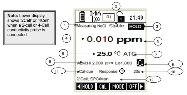
Figure 37 : Salinity measurement screen
