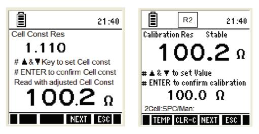
Figure 40 : Resistivity Cell constant & resistivity calibration
