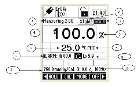
Figure 49 : Percentage saturation measurement screen
