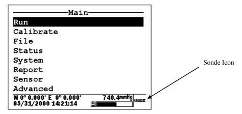
Note that the icon in the lower right of the screen has changed from "meter" to "sonde" indicating that the menu shown originates in the 6-series sonde. Note also that the 650 display has been designed to be very similar to that presented on a monitor when a 6-series sonde is attached to a PC as shown below.
