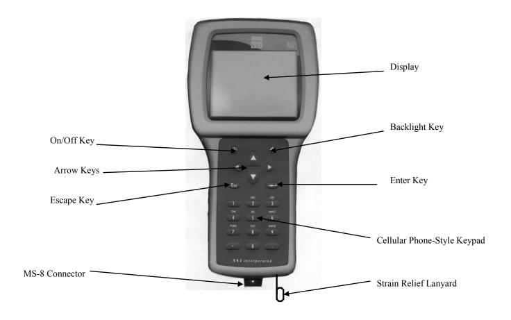
Note that the YSI 650 keypad consists of 20 keys as shown in the diagram above. There are four function keys, up, down, right and left arrow keys and an alpha/numeric keypad. The top left key that has a green circle and line, , is the ON/OFF key. The top right key, , activates the display backlight. The **Escape** key is labeled is the **Enter** key.
