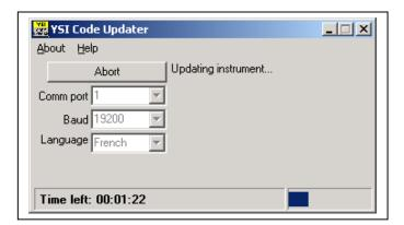
• When the update is finished (indicated on the PC screen as shown below), close the YSI Code Updater window (on the PC) by clicking on the "X" in the upper right corner of the window.
