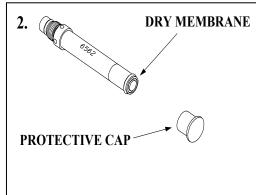
The DO membrane can be installed with the DO probe either free or installed in the sonde. Both methods are described in detail below. CAUTION: If you install the membrane with the probe not installed in the sonde, be sure that the protective cap is installed on the probe end away from the sensor face to ensure that the connector is not contaminated with electrolyte.
