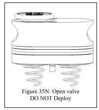
Lightly lubricate the o-rings on the outside of the battery cover. DO NOT lubricate the orange internal oring.
