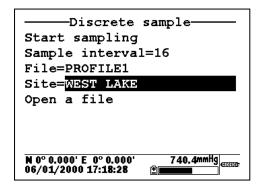
The user then highlights **Start sampling** and lowers the instrument into the water to begin the study. The data displayed on the screen is updated every 16 seconds. The user then highlights the **Start logging** selection in the sonde logging window in the upper right of the display and presses **Enter** to begin logging data to sonde memory. The message in the sonde logging window changes to **Stop logging**, indicating that logging has successfully been activated.
