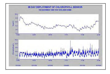
Note also that your may observe less or more noise at your site with no compromise in sensor performance. Occasional spikes during a monitoring study are normal and usually simply indicate the transient passage of a large phytoplankton particle over the optical face during the time of sampling.
