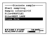
At the end of the 90 minute profile determination, the user either confirms the **Stop logging** command by pressing **Enter** or simply presses the **Escape** key to return to the sonde **Discrete sample** menu, highlights the **Close file** selection, and confirms the file closing by pressing **Enter**.
