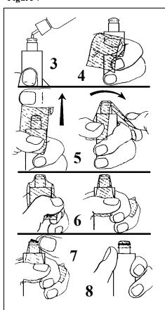
**NOTE**: You may find it more convenient to mount the probe vertically in a vise with rubber jaws while applying the electrolyte and membrane to the sensor tip.
