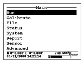
The user then selects **Run** from the sonde Main menu and **Discrete sample** from the **Run** menu, pressing **Enter** to confirm each selection.
