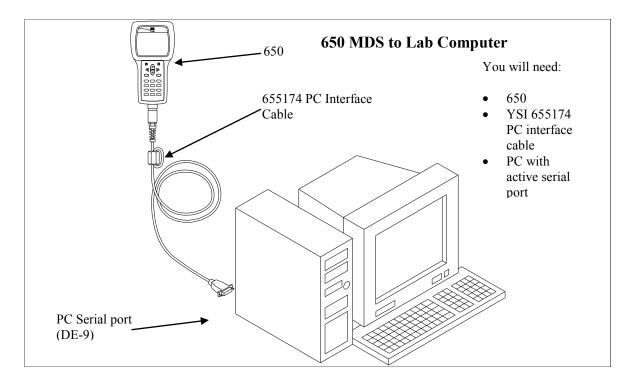
A sonde or 650 display/logger must be connected to one of the serial communication ports on the back of your PC. These ports are usually referred to as COM1, COM2, etc. Most computers have at least two COM ports but they are often not labeled. To identify a COM port, look for unused 9 or 25 pin, D-shaped connectors with pin contacts.
