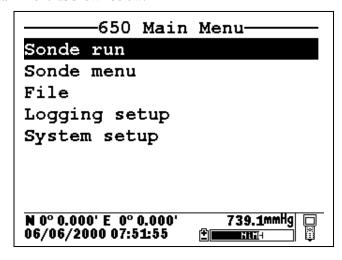
Using the arrow keys, highlight the **Sonde run** entry in the Main 650 Menu and press the **Enter** key. Readings from the 6-series sonde sensors will appear on the 650 Main Display in real-time as shown in the following diagram.
