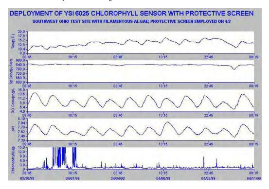
The flexible algal strands can become attached to the wiper arm and sometimes are resident on the probe optics even after a cleaning cycle. The key to decreasing the spiking effect is to minimize the free algae, which is present in the probe compartment of the sonde. This can sometimes be accomplished by encasing the sonde guard in standard fiberglass window screen wire which is available at most hardware stores and then anchoring the screen with rubber bands as shown in the picture below.
