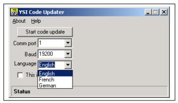
• Set the Comm port number to match the port to which you connected the sonde cable and make sure that the "This is an ADV6600" selection is NOT checked.
