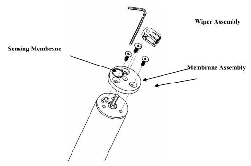
Note: The following steps can be carried out with the probe either installed in the sonde or removed from it. Avoid touching the sensing membrane (shown in the above drawing) during the procedure.
