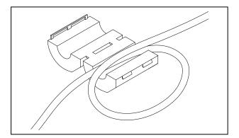
• Snap the two pieces of the bead together making certain that the tabs lock securely.
