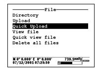
After the sonde file has been uploaded to the 650, the data is resident in the flash memory of both sonde and 650. Note that, if you choose to upload files from the sonde in CDF or ASCII format, the files will be characterized by a .txt extension in the 650 Directory and will NOT be viewable on the 650 display. To view the files, you must first transfer them from the 650 to your PC and then open them in a spreadsheet.
