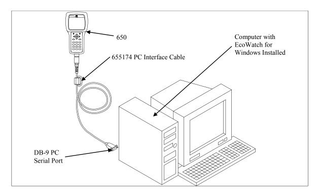
After the connection is made, run EcoWatch for Windows, click on the sonde icon in the upper toolbar, and set the Comm port number to match your interface. After this setup procedure, the following screen will be present on your PC monitor:
