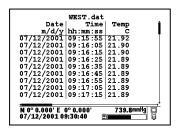
Note that, using these same basic guidelines, data could have been logged at another site on the same day with the user inputting a different site designation (file name and site name) in the field. Data could also have been logged single points or as a continuous data stream at each site simply by the choice of **Log single point** or **Start logging**, respectively, in the 650 Logging window.
