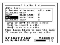
The two inserted entries can be moved either up or down in the list by highlighting them and pressing the **Up or Down arrow** key while holding down the **Enter** key or completely deleted by highlighting the entry and pressing the **Left arrow** key while holding down the **Enter** key as shown below.
