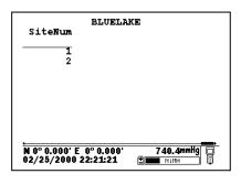
Note that the data from two sites is identified by the **Site Number** attached to each data record. To index these numbers to the appropriate locations, the user must consult the **Site list** by activating **Edit site list** from the **650 Logging setup** menu. The correlation between site names and numbers is found here, indicating that Site 1 is WEST and Site 2 is EAST.
