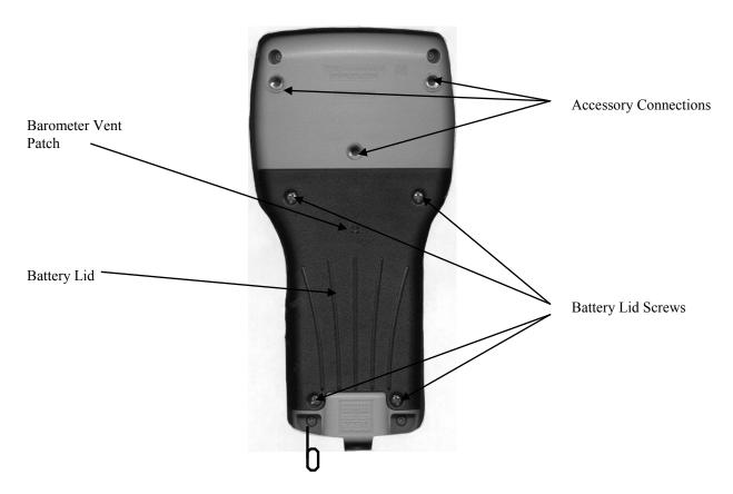
Note that the back of the case contains the battery lid that is attached to the main case with four captive screws and has three fittings for attachment of the ultraclamp and tripod accessories. In addition, the battery lid has a hole that is covered with water-impermeable patch for venting of the optional barometer.
