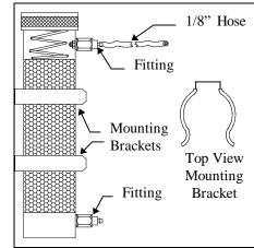
5. Remove the plug from the top fitting of the canister. Remove the plug from the barbed fitting on the end of the cable. Using the tubing provided in the kit, connect the canister to the fitting on the end of the cable. Remember to remove the remaining plug from the canister when ready to begin sampling. When putting the sonde into service, remove the plug to ensure that the sensor in the sonde is vented to the atmosphere.
