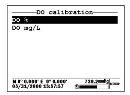
Use the 650 numeric entry keys and the right/left arrow keys to enter the current local barometric pressure. Then, press the **Enter** key and observe the dissolved oxygen reading until stabilization occurs. Make sure the **Calibrate** selection is highlighted in upper window.
