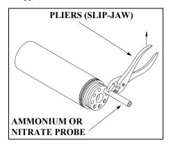
module is removed from the sonde, be sure to dry the sonde port and probe connector with compressed air and apply a very thin coat of lubricant to the O-ring before re-installation.
