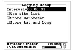
Press Enter at the highlighted **Interval** selection and use the arrow keys to scroll to the right and change the interval from 1 second to 10 seconds. Confirm the selection by pressing **Enter** and then press **Esc** to return to the **650 Main menu**.
