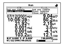
The user places the sonde in the water and then highlights the **Start logging** selection in the 650 logging window (upper left) and presses **Enter**. The user is then prompted to enter a **Filename and Site description** for the study as shown below.
