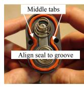
2. Press two of the outermost retaining tabs down into the groove. It should be clear that the retaining tabs have recessed into the groove along with the seal so that the tabs outermost edges are at or below the battery lid's mounting surface.
