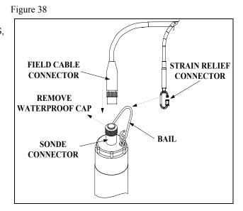
A built-in "key" will ensure proper pin alignment. Rotate the cable gently until the "key" engages and then tighten the connectors together by rotating clockwise. Attach the strain relief connector to the sonde bail. Rotate the strain relief connector nut to close the connector's opening.
