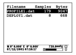
Note that the size of the file is shown in two different ways: (1) the number of samples (logged data points of several parameters) and (2) the total number of bytes of memory occupied by the file. Highlight the top file (PROFILE1) and press **Enter** to generate a display of the details of this file. Press **Escape** and then highlight the second file (DEPLOY1) and press **Enter** to again display information about the file.
