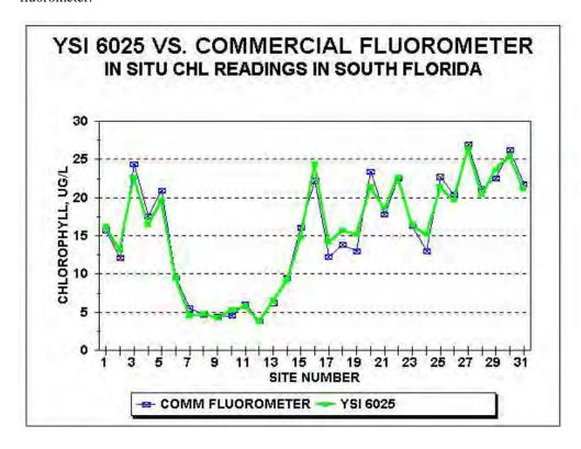
It is important for the user to remember that, because of the limitations defined in this appendix and in **Section 5, Principles of Operation**, YSI is unable to quote an accuracy specification for the *in vivo* measurement of chlorophyll.
