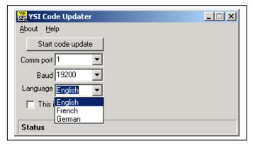
• Set the Comm port number to match the port to which you connected the sonde cable and make sure that the "This is an ADV6600" selection is NOT checked. Next, select the language (English, French, or German) which will be used in the menus of your sonde.
