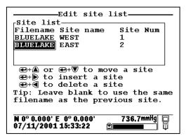
Note that the keystrokes for editing the site list are shown in the bottom of the Main Display. Thus, to insert (add) a file above the present cursor position, simply highlight the proper entry and press the **Right arrow** key while holding down the **Enter** key as shown in the following example. Note that two sites were inserted in the initial site list using this method.
