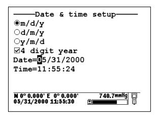
Enter the proper number from the keypad for the first date digit. Note that when you release the key, the cursor moves automatically to the next number. Repeat this process until the date is correct. Then press **Enter** to confirm the Date entry. Note also that, as described above, since alpha characters are inappropriate for this entry, only numeric entry is possible.
