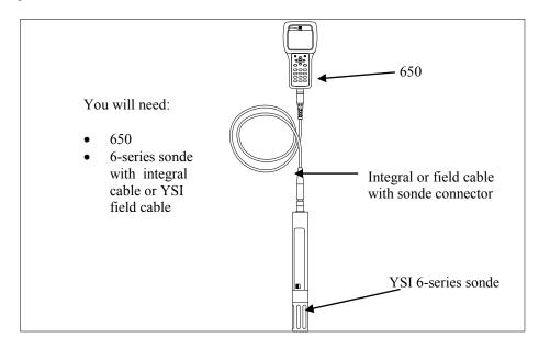
Figure 2. 650 interfaced to a 6-series sonde with user-supplied GPS.
