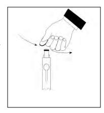
After completing the sanding procedure, repeatedly rinse the probe face with clean water and wipe with lens cleaning tissue to remove any grit left by the sanding disk. After cleaning, thoroughly rinse the entire tip of the probe with distilled or deionized water and install a new membrane.
