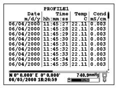
Use the arrow keys to scroll vertically to view more data points with regard to time or horizontally to view more sensor data within a particular data entry. The vertical and horizontal scroll bars identify your location within the data file.
