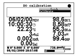
When the dissolved oxygen reading is stable, press the **Enter** key to confirm the calibration as indicated by the message "Calibrated" in the header. In addition, the message in the upper window will change from
