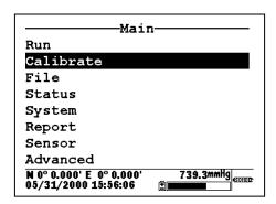
Use the arrow keys to highlight the **Dissolved Oxygen** selection and press **Enter**. Then, Use the arrow keys to highlight the **DO%** selection and press **Enter**.
