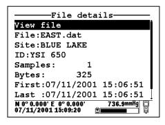
These files will remain "open" in 650 memory so that you can return to each location at a future time and log more data to the file designations WEST and EAST (but see note below). The key for this **Site list** setup is that all data logged will be stored in a separate file for each location (WEST and EAST) which were designated as file names at the site BLUE LAKE.
