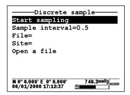
To set up the desired study parameters, the user uses the 650 keypad to change the Sample interval from 0.5 seconds to 16 seconds and inputs custom file (PROFILE1) and site (WEST LAKE) designations.
