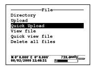
Select the **Upload** or **Quick upload** (last file) and press **Enter**. Then follow the instructions including selection of file format – YSI recommends the PC6000 format. Press **Enter** and the display will indicate that upload of data from sonde to 650 is in progress as shown below. When the upload is complete, the display will return to the **Sonde File** menu.
