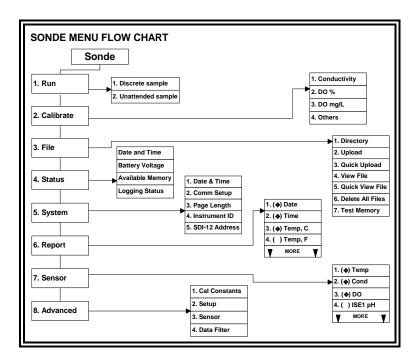
**NOTE:** When using the 650, <u>all</u> sonde functions are accessed through the **Sonde menu** prompt. These include:
