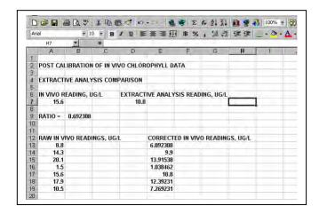
Note: Be sure to carry out1-point calibration of the sensor before the study, using deionized water to make certain that the sensor reads zero in chlorophyll-free water.
