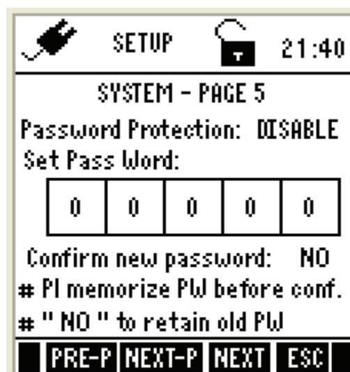
When you enable password protection, the meter prompts you to enter the password whenever you try to access the Setup or Calibration mode. The meter does not allow you to edit setup parameters or perform a new calibration unless you enter the correct password. If an incorrect password is entered for 3 consecutive times, the meter goes to measurement mode.
