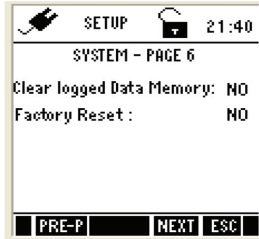
This allows you to clear the memory and reset the meter to factory defaults.
