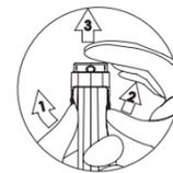
Fig. 1: Removing battery cover
