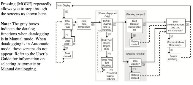
**Note:** The gray boxes indicate the datalog functions when datalogging is in Manual mode. When datalogging is in Automatic mode, these screens do not appear. Refer to the User's Guide for information on selecting Automatic or Manual datalogging.
