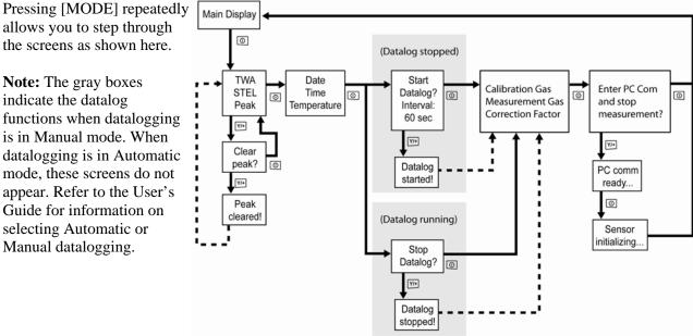
**Note:** The gray boxes indicate the datalog functions when datalogging is in Manual mode. When datalogging is in Automatic mode, these screens do not
