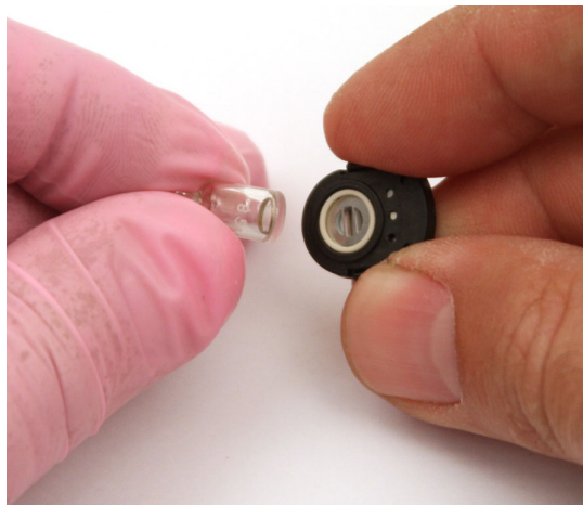
Figure 33: Reinstalling the Electrode Lamp
