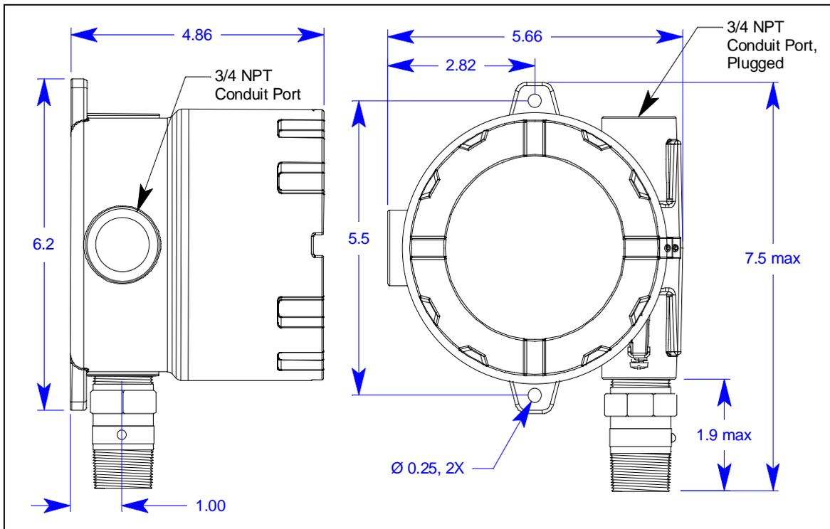
**Figure 16: Outline & Mounting Dimensions, IR Combustible, CO<sub>2</sub>, and MPS LEL Detectors**
