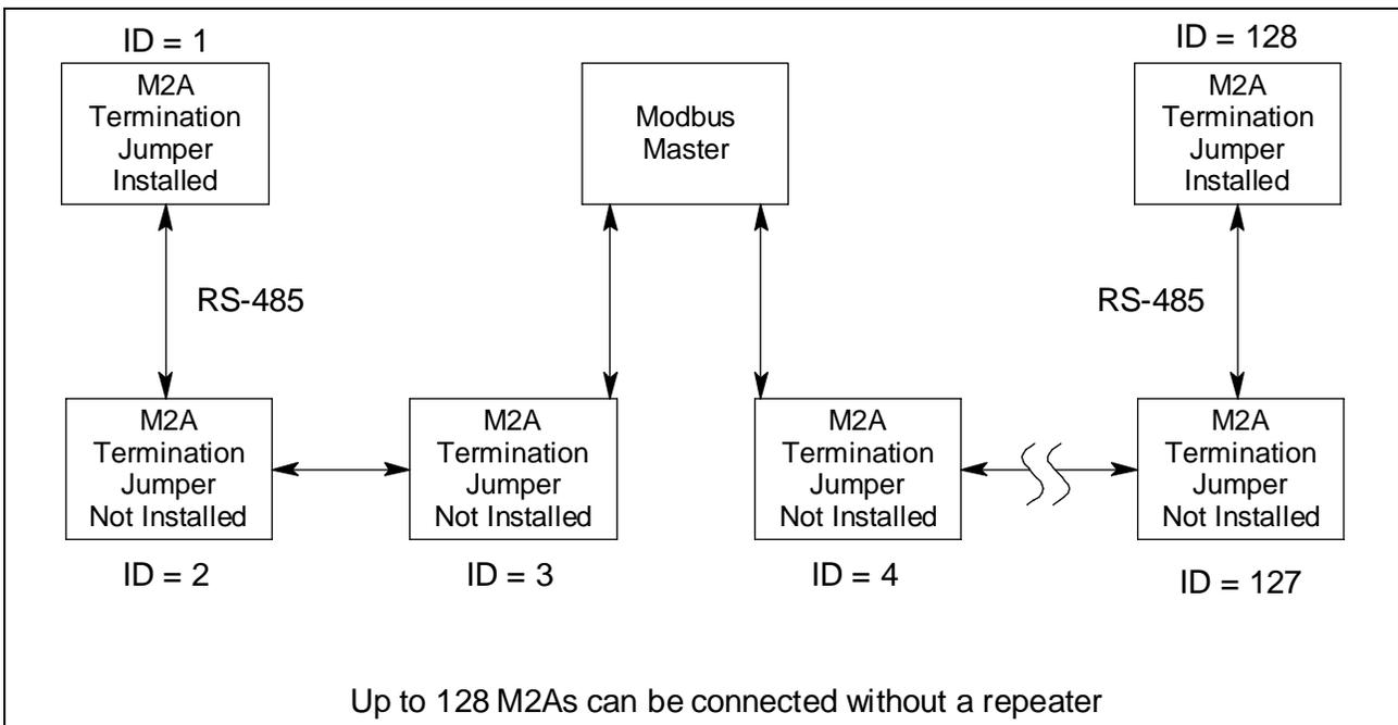
Figure 36: Multiple M2As in a Two Branch Configuration
