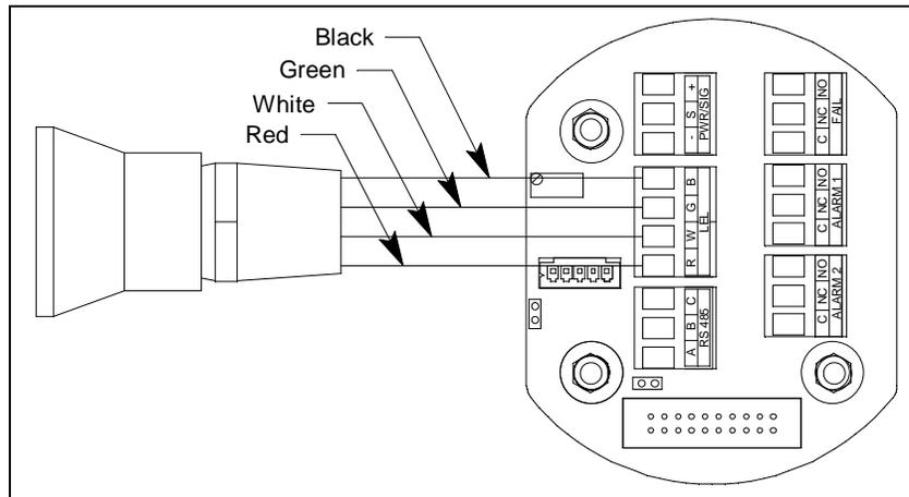
Figure 22: Catalytic LEL and ppm Detector Wiring
