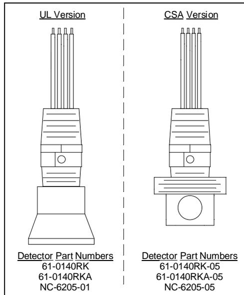
**Figure 2: Catalytic Sensors**
