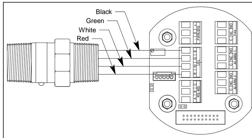
Figure 23: IR Combustible/IR CO<sub>2</sub>/MPS LEL Detector Wiring
