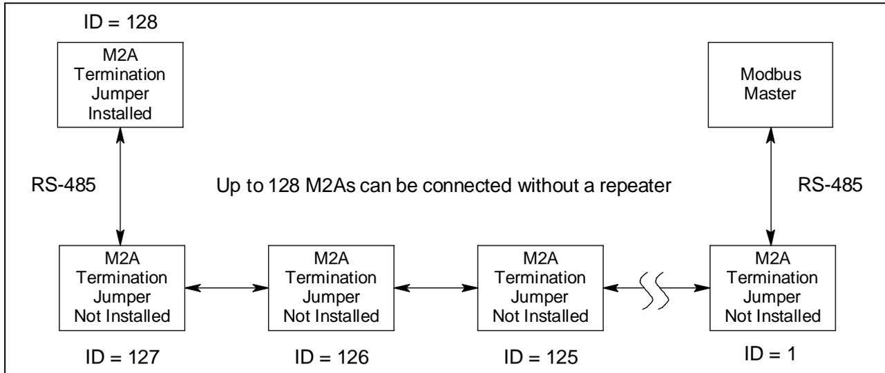
Figure 35: Multiple M2As in a Daisy Chain Configuration
