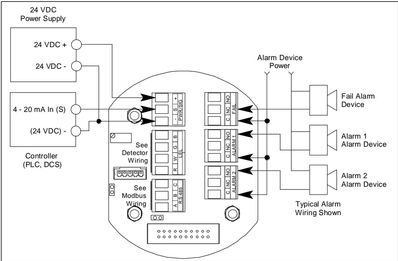
**Figure 37: PLC and DCS Device Wiring**
