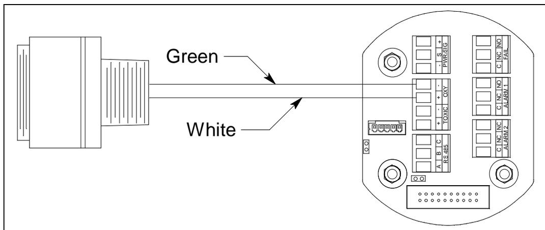
**Figure 26: Capillary Type Replaceable Sensor Oxygen Detector Wiring**
