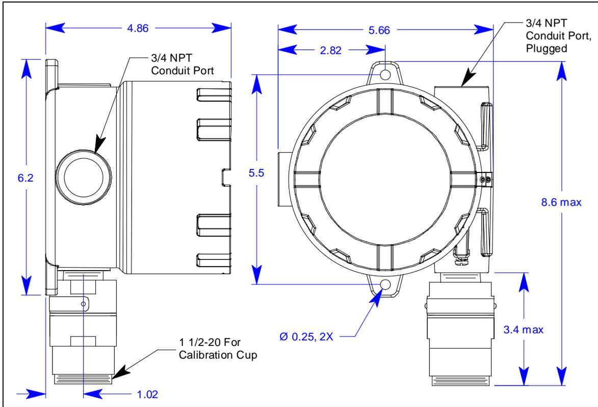
**Figure 19: Outline & Mounting Dimensions, H<sub>2</sub>S, CO, HCN, and Oxygen, CSA, Explosion-Proof**
