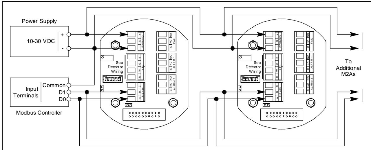
Figure 34: Alternate Modbus Wiring
