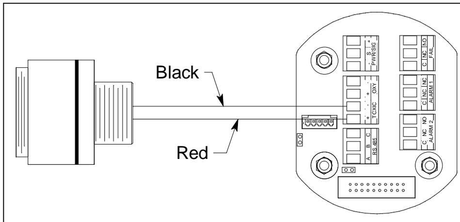
Figure 28: H<sub>2</sub>S/CO Detector Wiring
