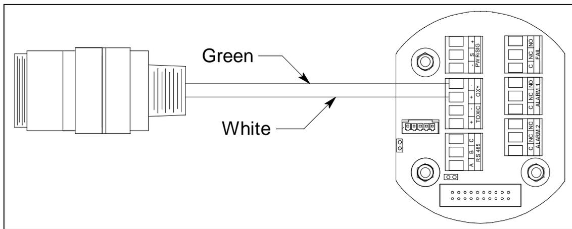
**Figure 25: CSA Capillary Type Oxygen Detector Wiring**
