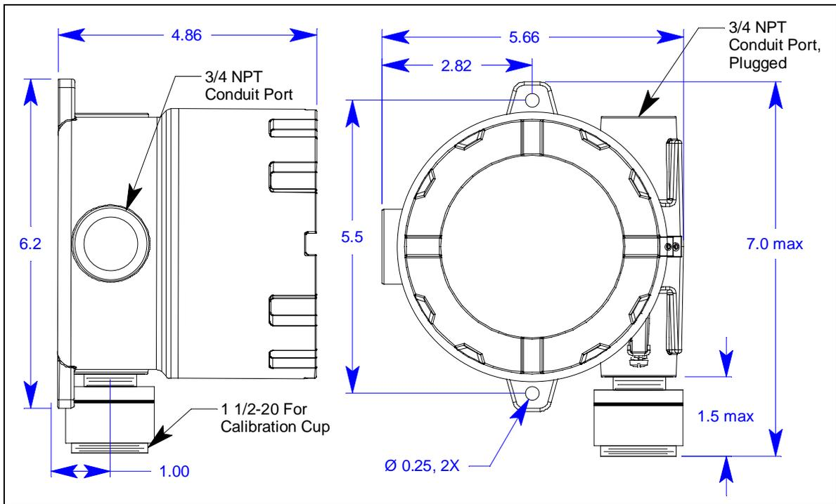
**Figure 18: Outline & Mounting Dimensions, Replaceable Sensor, H<sub>2</sub>S, CO, and Oxygen, Non-Explosion Proof**
