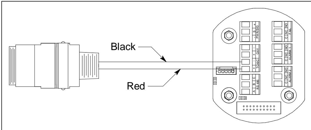
Figure 27: H<sub>2</sub>S/CO/HCN Detector Wiring, CSA
