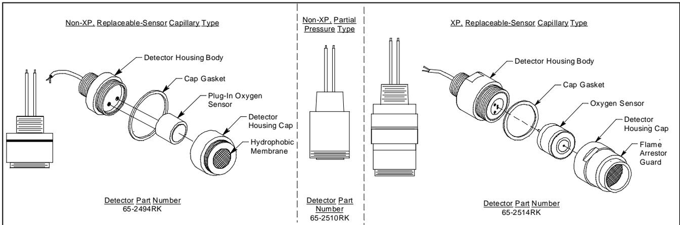
**Figure 4: Oxygen Detectors**
