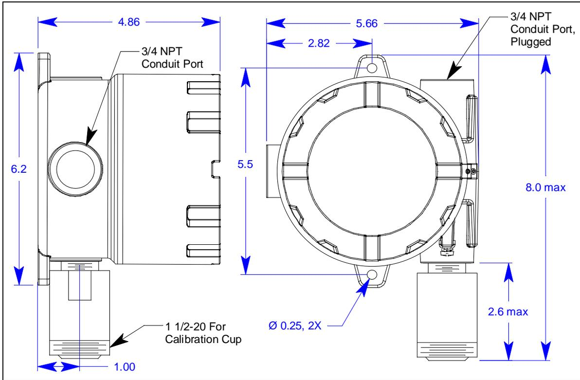
**Figure 17: Outline & Mounting Dimensions, Oxygen, Partial Pressure Type**
