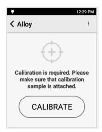
If this is the first time the unit is being used (or the first time the unit being used for the day), the unit will need calibrating.
