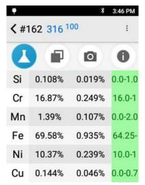
Specifications column lists the specification of the best alloy grade match for the determined chemistry of the sample.
