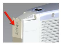
Place the 316 coupon that came with the unit on the nose.
