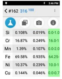
The first column on the left lists all detected elements. Scroll down to see additional elements.
