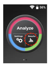
The default screen will list all of the tests taken on the instrument.
