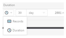
When set by number of records the time of the recording phase will be displayed detailing how long that phase will run. When set by time, the total number of records for that phase will be displayed.
