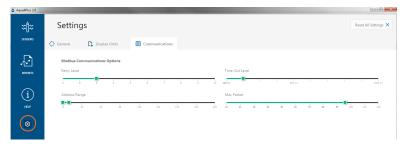
Simply drag the Address Range slider higher up to increase the maximum Modbus address scanned. If you've scanned all the way up through address 255 and still have no connection click Troubleshooting for further troubleshooting or contact Seametrics Tech Support for assistance.
