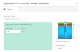
Aqua4Plus 2.0 will take 10 measurements and display the average. Watch for stability while the software is measuring to ensure an accurate calibration.
