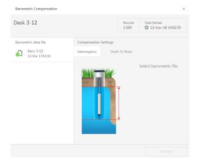
If compensating for Depth to Water enter your depth to water reference measurement and the date/time the measurement was taken (typically taken with a water level indicator before data is uploaded from the sensor) before clicking Continue.
