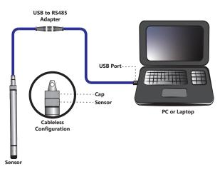
Connect the sensor to your PC using Seametrics' USB to RS485 adapter.
