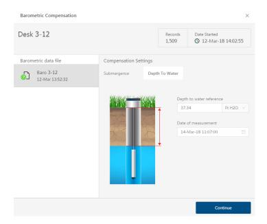
Aqua4Plus 2.0 will perform the barometric compensation and create a new compensated report. Original reports are retained as uploaded.
