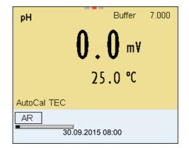
13 Wait for the measurement with stability control to be completed or terminate the stability control and take over the calibration value with **<ENTER>**.
