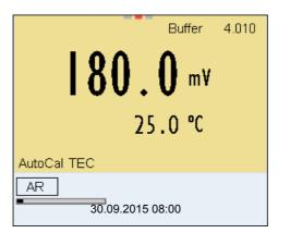
19 Wait for the measurement with stability control to be completed or terminate the stability control and take over the calibration value with **<ENTER>**.
