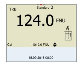
16 If necessary, terminate the calibration as a two-point calibration with **<M>**.
