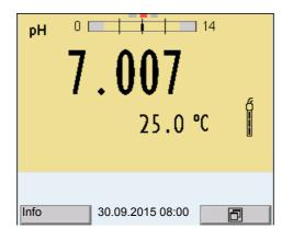
1 In the measured value display: Display the sensor data (sensor name, series number) with [*Info*].
