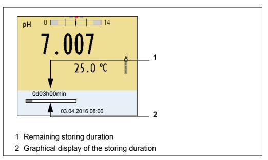
The active automatic data storing function can be recognized by the progress bar in the status line. The progress bar indicates the remaining storage duration.
