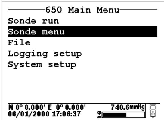
From the **650 Main Menu**, select **Sonde menu** and press **Enter**. A display similar (depending on sonde type and sonde software version) to that shown below will appear:
