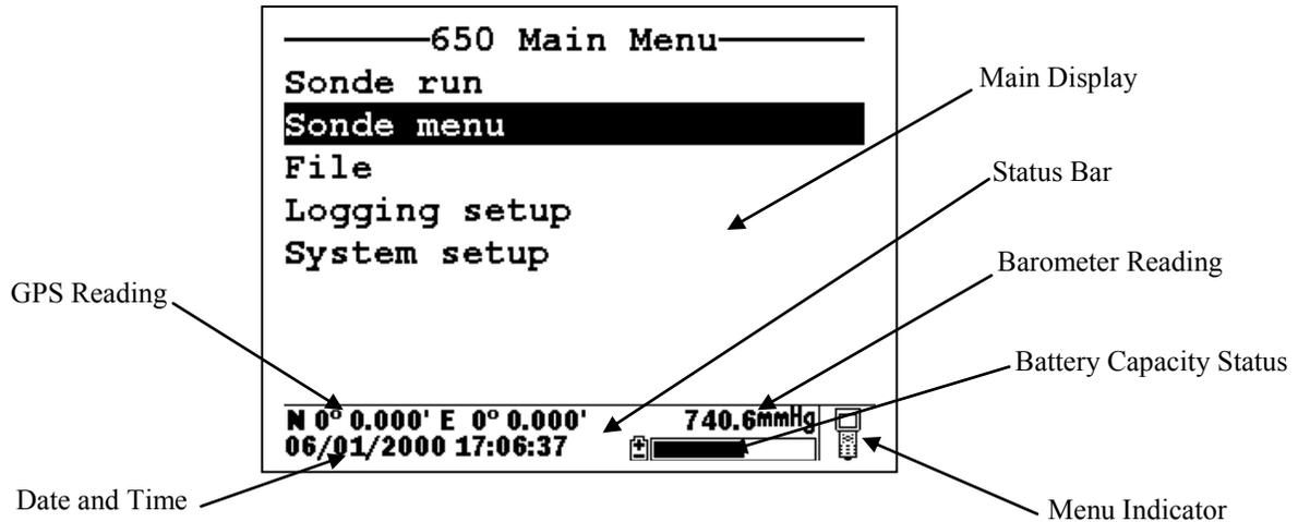
**2.10.1 Date and Time.** This is the date and time for the clock in the 650, set by the user from the **System setup** menu as described above. The date and time entries are updated in real-time in the Status Bar.
