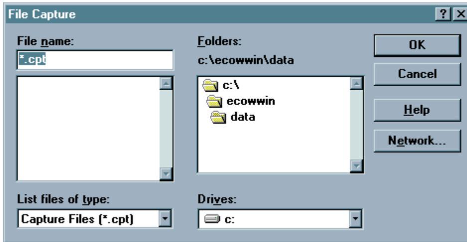
A common example is using a sonde in **Run Mode**. The sonde is simply taking readings and sending them to the COM port. If you want to keep a record of these readings, then a simple way to do so is to turn **Capture** on. When you are finished, run the **Capture** command again to turn it off.
