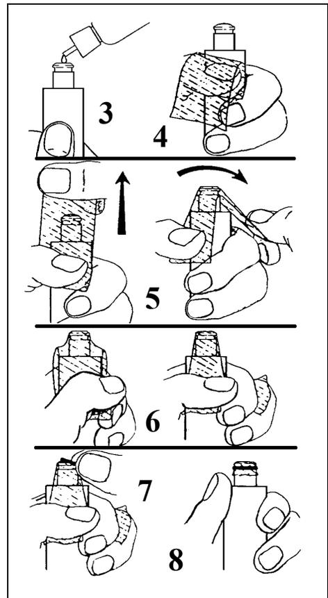
**NOTE:** You may find it more convenient to mount the probe vertically in a vise with rubber jaws while applying the electrolyte and membrane to the sensor tip.
