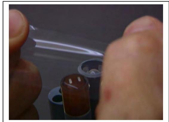
Hold the membrane so that all four corners are supported, but do not stretch the membrane laterally.
