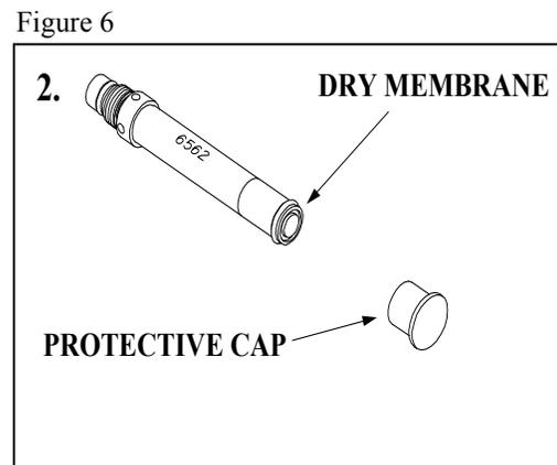
The DO membrane can be installed with the DO probe either free or installed in the sonde. Both methods are described in detail below. **CAUTION: If you install the membrane with the probe not installed in the sonde, be sure that the protective cap is installed on the probe end away from the sensor face to ensure that the connector is not contaminated with electrolyte.**
