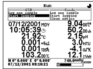
The user places the sonde in the water and then highlights the **Start logging** selection in the 650 logging window (upper left) and presses **Enter**. The user is then prompted to enter a **Filename and Site description** for the study as shown below.
