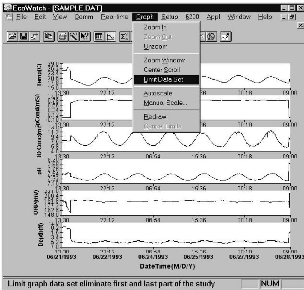
Figure 48 Using Limit Data Set to Display a Subset of Data
