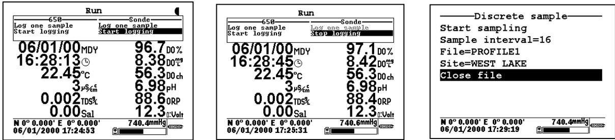
At the end of the 90 minute profile determination, the user either confirms the **Stop logging** command by pressing **Enter** or simply presses the **Escape** key to return to the sonde **Discrete sample** menu, highlights the **Close file** selection, and confirms the file closing by pressing **Enter**.
