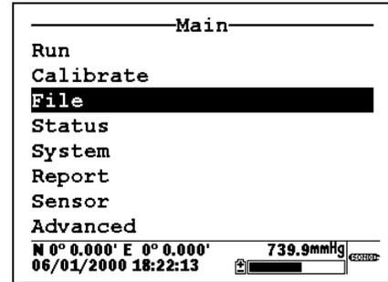
To view the data on return from the site, the user selects the sonde menu **File** selection, presses **Enter** to confirm the entry, and then highlights the **View file** selection and presses **Enter**. Following these instructions generates a display of the data that is stored in the sonde memory under the default name NONAME1. Use the right/left arrow keys to scroll horizontally to view all of the data.
