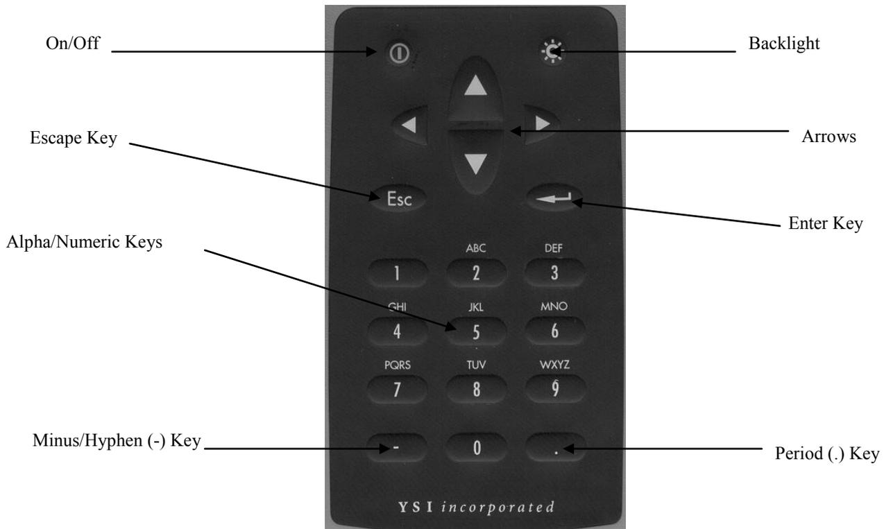
The 650 keypad allows the user to navigate various sonde and 650 menu selections and to make alpha/numeric entries into both the 650 and sonde software. The arrow keys are used to select various options in the menus; the cellular phone-style alpha/numeric keys allow data entry; the **Enter** key is used to confirm selections; and the **Escape** key returns the user to the previous position in the menu structure.
