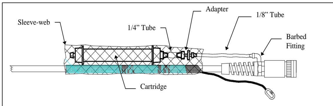
1. Place the short length of 1/4" tubing onto the 1/4" side of the 1/8" to 1/4" adapter fitting. Seat firmly.
