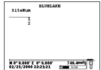
Note that the data from two sites is identified by the **Site Number** attached to each data record. To index these numbers to the appropriate locations, the user must consult the **Site list** by activating **Edit site list** from the **650 Logging setup** menu. The correlation between site names and numbers is found here, indicating that Site 1 is WEST and Site 2 is EAST.
