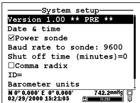
Use the arrow keys to highlight the **Date and Time** selection and press the **Enter** key. The following display will appear:
