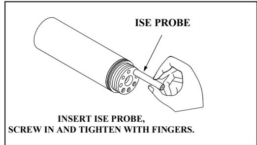
**IMPORTANT:** Make sure that the probe nut or probe body of the ISE probes are seated directly on the sonde bulkhead. This will ensure that connector seals will not allow leakage.
