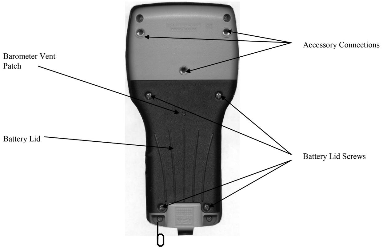
Note that the back of the case contains the battery lid that is attached to the main case with four captive screws and has three fittings for attachment of the ultraclamp and tripod accessories. In addition, the battery lid has a hole that is covered with water-impermeable patch for venting of the optional barometer.
