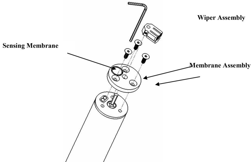
Note: The following steps can be carried out with the probe either installed in the sonde or removed from it. Avoid touching the sensing membrane (shown in the above drawing) during the procedure.
