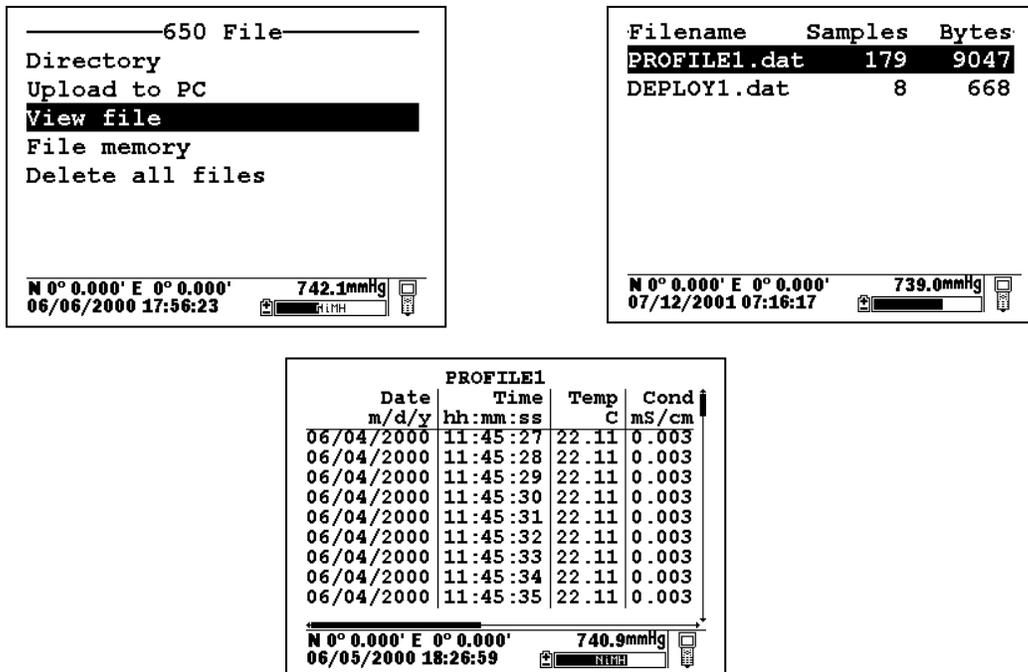
Use the arrow keys to scroll vertically to view more data points with regard to time or horizontally to view more sensor data within a particular data entry. The vertical and horizontal scroll bars identify your location within the data file.
