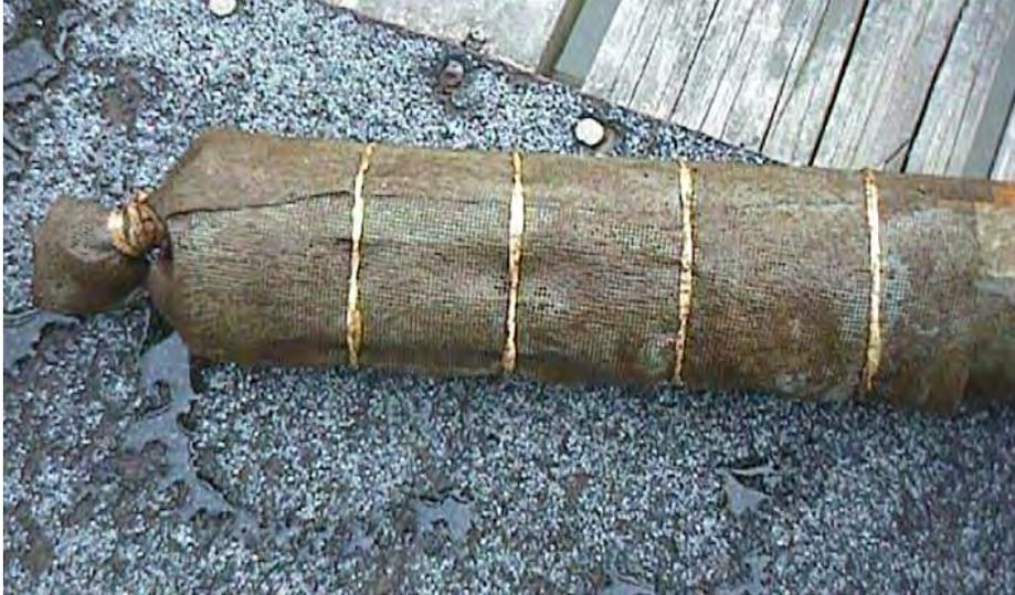
Note the significant improvement in the overall noise level of the readings after the screen was installed on 4/2/99. However, there is no guarantee that this solution will completely solve spiking problems caused by macro algal species. In some applications, it may be necessary to clean the sonde and probes at a frequent interval to minimize the number of erroneous readings.
