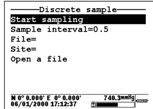
To set up the desired study parameters, the user uses the 650 keypad to change the Sample interval from 0.5 seconds to 16 seconds and inputs custom file (PROFILE1) and site (WEST LAKE) designations.
