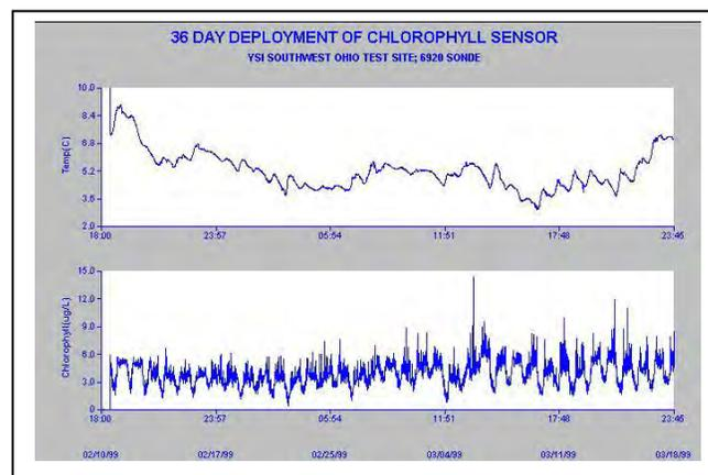
Note also that you may observe less or more noise at your site with no compromise in sensor performance. Occasional spikes during a monitoring study are normal and usually simply indicate the transient passage of a large phytoplankton particle over the optical face during the time of sampling.
