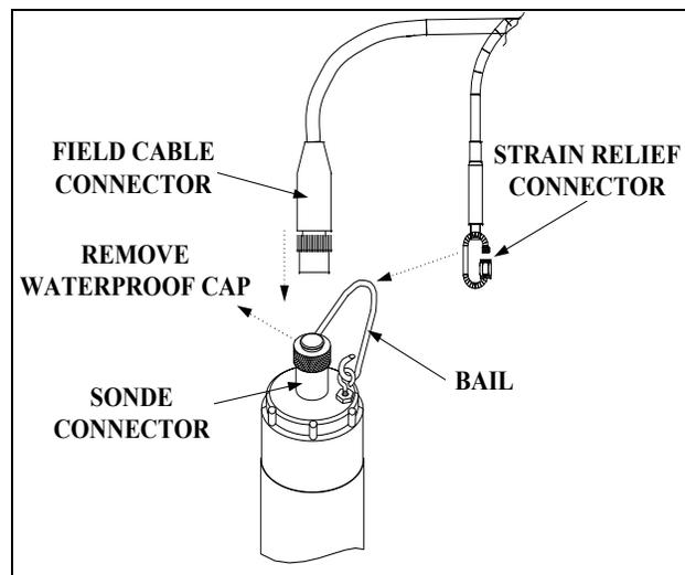
A built-in “key” will ensure proper pin alignment. Rotate the cable gently until the “key” engages and then tighten the connectors together by rotating clockwise. Attach the strain relief connector to the sonde bail. Rotate the strain relief connector nut to close the connector's opening.
