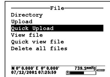
After the sonde file has been uploaded to the 650, the data is resident in the flash memory of both sonde and 650. Note that, if you choose to upload files from the sonde in CDF or ASCII format, the files will be characterized by a .txt extension in the 650 Directory and will NOT be viewable on the 650 display. To view the files, you must first transfer them from the 650 to your PC and then open them in a spreadsheet.
