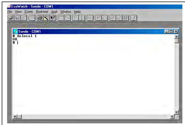
After taking the above action the parameter “DOsat %Local” or “ODOsat %Local”, depending on the type of DO sensor used in your sonde, will be present in your Report menu. If you want to remove the parameter, return to the “#” prompt, type “dolocal 0”, and press **Enter**.
