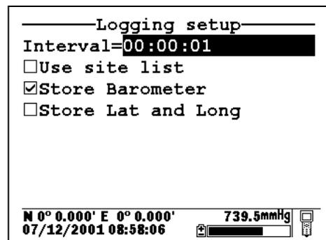
Press Enter at the highlighted **Interval** selection and use the arrow keys to scroll to the right and change the interval from 1 second to 10 seconds. Confirm the selection by pressing **Enter** and then press **Esc** to return to the **650 Main menu**.
