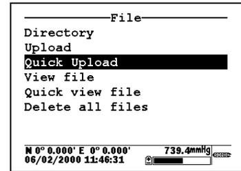
Select the **Upload** or **Quick upload** (last file) and press **Enter**. Then follow the instructions including selection of file format – YSI recommends the PC6000 format. Press **Enter** and the display will indicate that upload of data from sonde to 650 is in progress as shown below. When the upload is complete, the display will return to the **Sonde File** menu.
