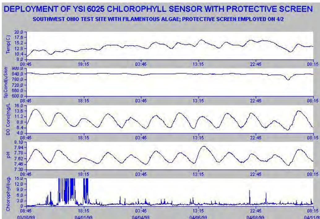
The flexible algal strands can become attached to the wiper arm and sometimes are resident on the probe optics even after a cleaning cycle. The key to decreasing the spiking effect is to minimize the free algae, which is present in the probe compartment of the sonde. This can sometimes be accomplished by encasing the sonde guard in standard fiberglass window screen wire which is available at most hardware stores and then anchoring the screen with rubber bands as shown in the picture below.
