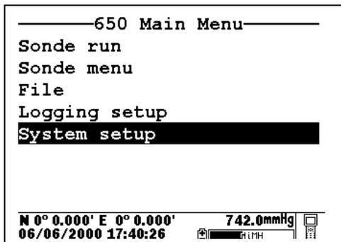
Use the arrow keys to highlight the **System setup** selection and press the **Enter** key. A display similar to the following will appear (Note that the exact format of your displays will depend on the software version):
