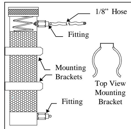
5. Remove the plug from the top fitting of the canister. Remove the plug from the barbed fitting on the end of the cable. Using the tubing provided in the kit, connect the canister to the fitting on the end of the cable. Remember to remove the remaining plug from the canister when ready to begin sampling. When putting the sonde into service, remove the plug to ensure that the sensor in the sonde is vented to the atmosphere.
