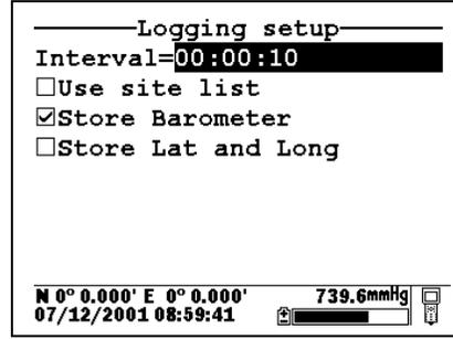
Once the sample interval is set correctly in the **650 Logging setup** menu, the user simply highlights the **Sonde run** selection in the **650 Main menu** and presses **Enter** to begin data display.
