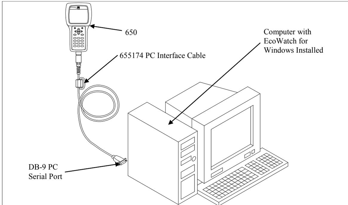
After the connection is made, run EcoWatch for Windows, click on the sonde icon in the upper toolbar, and set the Comm port number to match your interface. After this setup procedure, the following screen will be present on your PC monitor:
