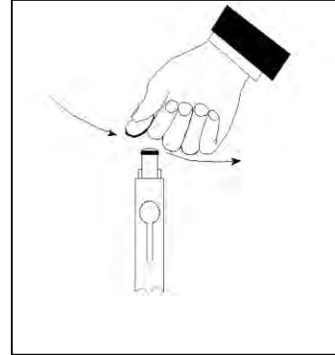
After completing the sanding procedure, repeatedly rinse the probe face with clean water and wipe with lens cleaning tissue to remove any grit left by the sanding disk. After cleaning, thoroughly rinse the entire tip of the probe with distilled or deionized water and install a new membrane.
