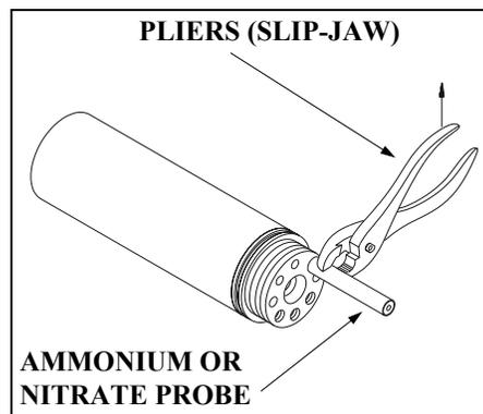
**NOTE:** The ion selective membranes are fragile. Be certain to: (1) Use only *moist*, high quality lens cleaning tissue for the cleaning procedure (not paper towels or other coarse materials); and (2) Stroke the probe face very gently with the tissue during the procedure. *If you do not adhere to these instructions, you can seriously damage the sensors.*
