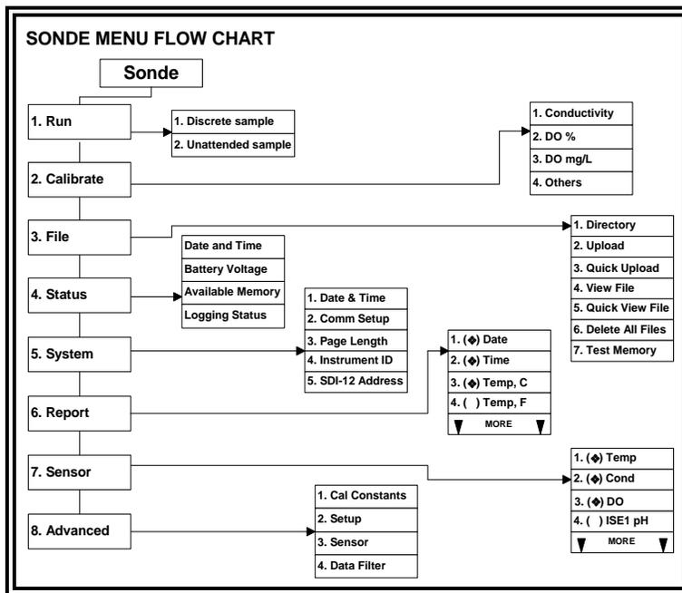
**NOTE:** When using the 650, all sonde functions are accessed through the **Sonde menu** prompt. These include:
