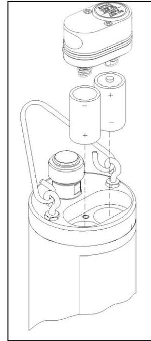
Install 8 C-size alkaline batteries according to the following directions and Figure 35.
