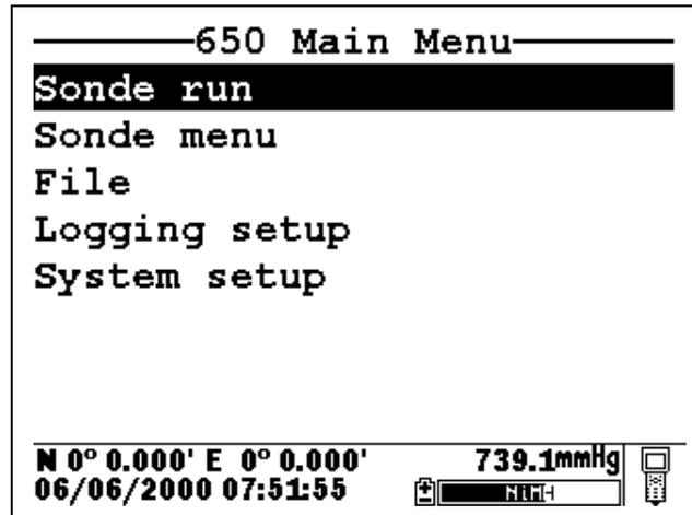
Using the arrow keys, highlight the **Sonde run** entry in the Main 650 Menu and press the **Enter** key. Readings from the 6-series sonde sensors will appear on the 650 Main Display in real-time as shown in the following diagram.
