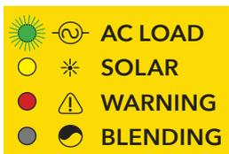
If the motor is properly connected, the Blender 2500 will move to the startup procedure. The green AC LOAD LED (See Figure 23: LED 1 - AC Load Is On) will have a solid green light and the motor will start running. The Blender 2500 immediately performs MPPT operation over the solar PV input to offset AC source power.
