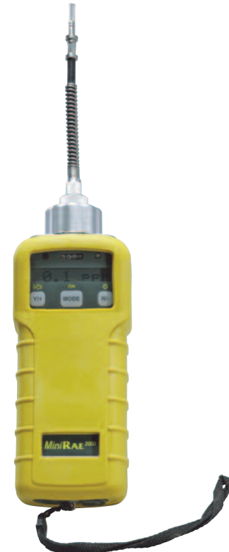
MiniRAE 2000 Photoionization Detector
