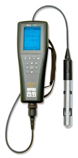
The ProODO is a digital signal instrument. Any ProODO cable can be connected and used on any ProODO instrument. The luminescent optical probes hold the calibration information internally.
