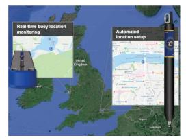
**Continuous GPS** – HydroVu uses VuLink's GPS to automatically locate and mark devices on maps, syncing devices and locations, increasing data quality, and making it easier to track free-floating buoys.
