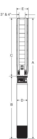
NOTES: Models 2-15 Stgs. are suitable for use in 6" (15 cm) wells, 16-18 Stgs. are suitable for use in 8" (20 cm) wells.
