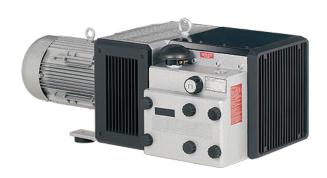
The vacuum and pressure flows are free of pulsation because the inlet and outlet ports do not have valves and the air is moved continuously rather than intermittently.
