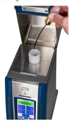
The CTX™ 500S model is readyto-go factory calibrated to comply with MARPOL regulations for sulfur in fuel oil testing.
